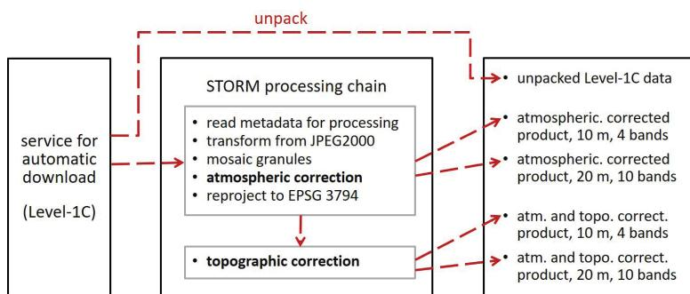
Figure 1: Implemented workflow for processing Sentinel-2 data of Slovenia.
