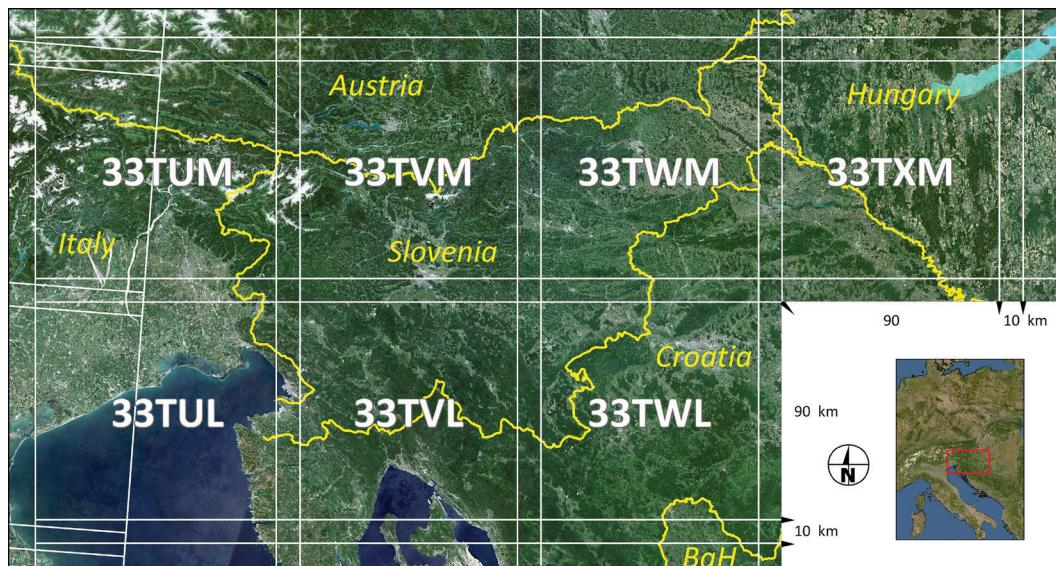
Figure 2: In ESA Sentinel-2 tiling grid Slovenia is covered by seven  $110 \times 110$  km<sup>2</sup> tiles in UTM 33 North zone (33TUM to 33TWL). Background image for small overview image is taken from European Environment Agency (EEA).
