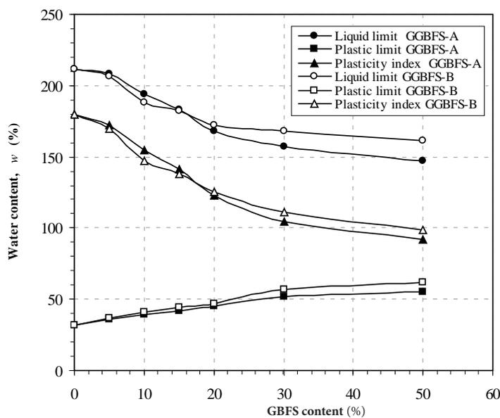
Figure 6. Effect of GGBFS on the consistency parameters of Bentonite clay.
