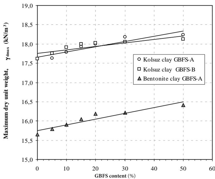
Figure 11. Effect of GGBFS on the maximum dry unit weight of clayey soils.
