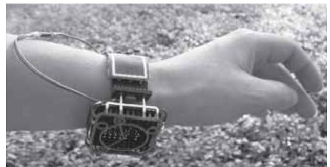
Fig. 7: Thermoelectric bracelet plus flex on which the radio and the sensor electronic are implemented.
