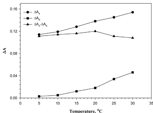
**Figure 8.** Effect of temperature. Conditions:  $\text{SCN}^-$ ,  $1.2 \mu\text{g mL}^{-1}$ ;  $\text{HCl}$ ,  $0.050 \text{ M}$ ;  $\text{MCP}$ ,  $2.34 \times 10^{-3}$ ;  $\text{KBr}$ ,  $2.0 \times 10^{-3} \text{ M}$  and  $\text{NaIO}_4$ ,  $3.0 \times 10^{-3} \text{ M}$ .
