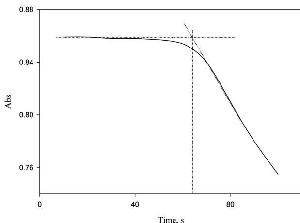
**Figure 9.** Graphical estimation of reaction induction period.
