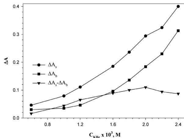
**Figure 6.** Effect of KBr concentration. Conditions: Fe(II), 0.20  $\mu\text{g mL}^{-1}$ ;  $\text{SCN}^-$ , 1.2  $\mu\text{g mL}^{-1}$ ; HCl, 0.050 M; MCP,  $2.6 \times 10^{-6}$  M;  $\text{NaIO}_4$ ,  $5.0 \times 10^{-3}$  M and temperature of 20  $^\circ\text{C}$ .
