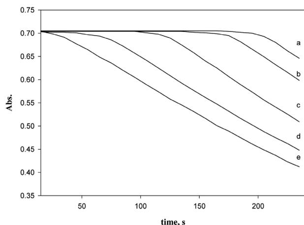
**Figure 2.** Absorbance change profile. Conditions: same as Fig. 1 with  $\text{Fe(II)}$  concentrations of (a) 0.00, (b) 0.030, (c) 0.20, (d) 1.0, (e)  $3.0 \mu\text{g mL}^{-1}$ .
