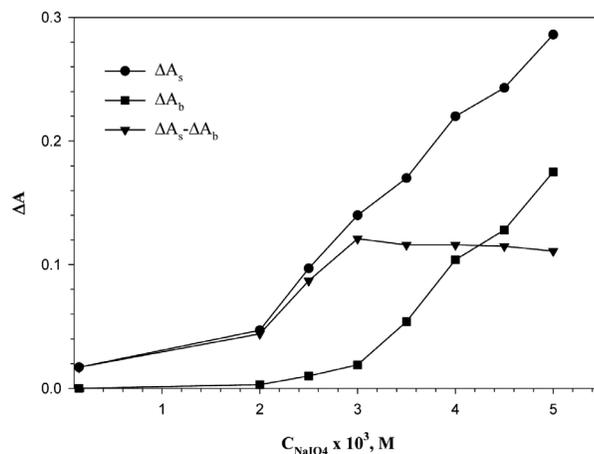
**Figure 7.** Effect of  $\text{NaIO}_4$  concentration. Conditions: Fe(II), 0.20  $\mu\text{g mL}^{-1}$ ;  $\text{SCN}^-$ , 1.2  $\mu\text{g mL}^{-1}$ ; HCl, 0.050 M; MCP,  $2.6 \times 10^{-6}$  M; KBr,  $2.0 \times 10^{-3}$  M and temperature of 20  $^\circ\text{C}$ .
