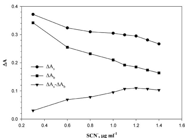
**Figure 5.** Effect of  $\text{SCN}^-$  concentration. Conditions: Fe(II), 0.20  $\mu\text{g mL}^{-1}$ ; HCl, 0.050 M; MCP,  $2.6 \times 10^{-6}$  M; KBr,  $2.0 \times 10^{-3}$  M,  $\text{NaIO}_4$ ,  $5.0 \times 10^{-3}$  M and temperature of 20  $^\circ\text{C}$ .
