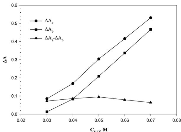
**Figure 4.** Effect of HCl concentration. Conditions: Fe(II), 0.20  $\mu\text{g mL}^{-1}$ ;  $\text{SCN}^-$ , 1.0  $\mu\text{g mL}^{-1}$ ; MCP,  $2.6 \times 10^{-5}$  M; KBr,  $2.0 \times 10^{-3}$  M,  $\text{NaIO}_4$ ,  $5.0 \times 10^{-3}$  M and temperature of 20  $^\circ\text{C}$ .
