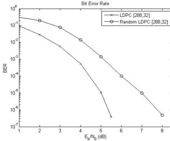
Figure 5: BER performance of the  $[288, 32, 56]$  LDPC code derived from the cubic semisymmetric graph with 576 vertices.
