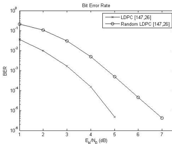
Figure 4: BER performance of the  $[147, 26, 26]$  LDPC code derived from the cubic semisymmetric graph with 294 vertices.
