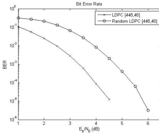
Figure 6: BER performance of the  $[448, 48, 100]$  LDPC code derived from the cubic semisymmetric graph with 896 vertices.
