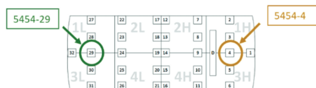
Figure 1: Scheme of the position of the as-cast sample 5454-29 and homogenized sample 5454-4 from the slice of the slab
