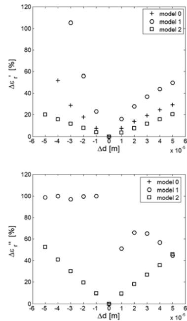
**Figure 3:** Error in real and imaginary component of permittivity in percentage as a function of an air gap for a frequency of 10GHz for titanium dioxide mixed with wax with different measurement set-up geometries.
