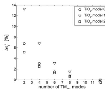
**Figure 7:** Error in real component of permittivity in percentage as a function of a number of  $TM_{0n}$  modes for a frequency of 10GHz for titanium dioxide mixed with wax with different measurement set-up geometries.
