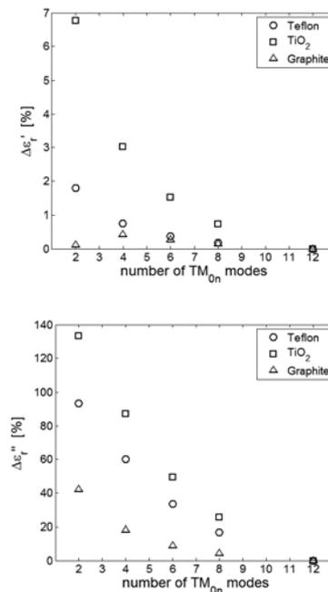
**Figure 6:** Error in real and imaginary component of permittivity in percentage as a function of a number of  $TM_{0n}$  modes for a frequency of 10GHz for different materials with measurement set-up geometry of model 0.
