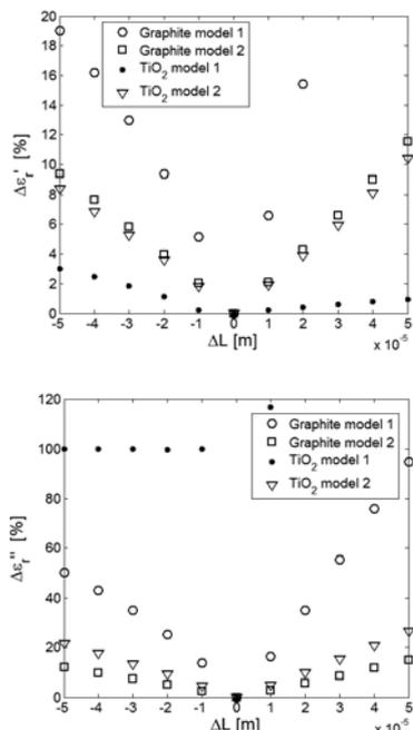
**Figure 5:** Error in real and imaginary component of permittivity in percentage as a function of the sample thickness for a frequency of 10GHz for titanium dioxide-wax and graphite-wax composites with different measurement set-up geometries.
