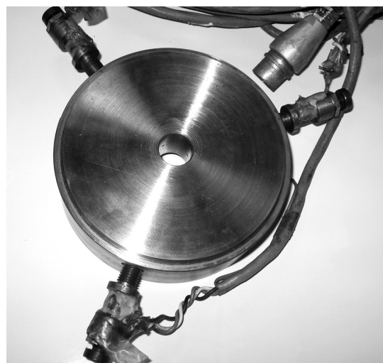
Figure 4: Experimental tool, receiver with three measuring pin load-cells Slika 4: Eksperimentano orodje: prejemnik s tremi merilnimi trni
