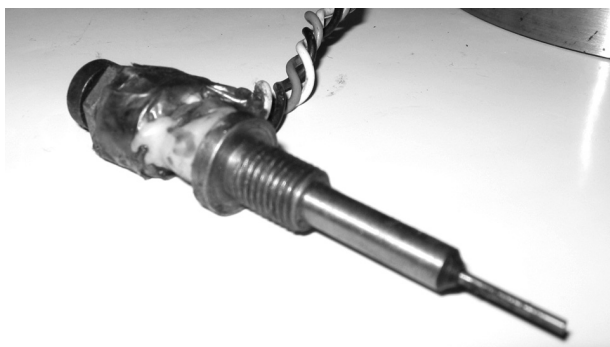
Figure 2: Measuring pin load-cell for radial forces Slika 2: Merilna celica s trni za radialne sile
