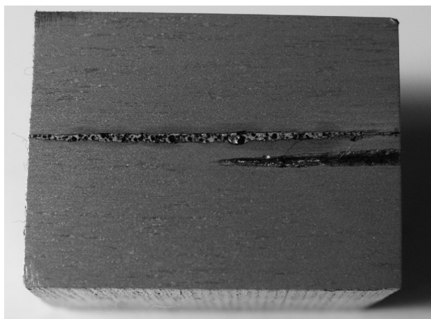
Figure 12: Forging No. 447 660. Macro-shape of the sample at the place of defect location.
