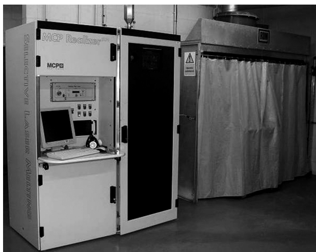
Figure 8: SLM system – Realiser MTT-Group, UK
