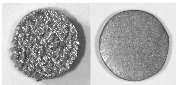
Figure 7: Test samples obtained by SLM (left) and by vacuum casting (right)
