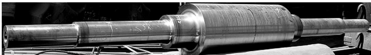
Figure 10: Defective generator rotor shaft – forging No. 447 660
