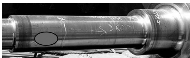
Figure 11: Detail of extent and location of the defect on the generator rotor shaft – forging No. 447 660
