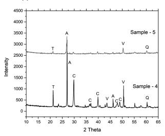
**Figure 7:** XRD of the wall samples: C: calcite, A: aragonite, V: vaterite, P: portlandite, T: tobermorite, Q: quartz
