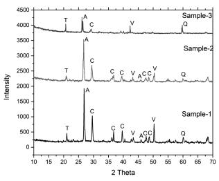
**Figure 6:** XRD of the roof samples: C: calcite, A: aragonite, V: vaterite, P: portlandite, T: tobermorite, Q: quartz
