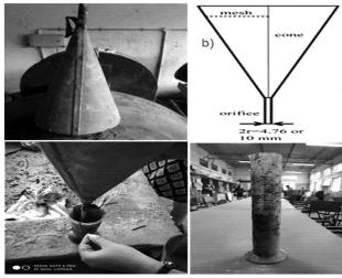
Figure 10: a), b), c) Marsh-cone test; d) stability
