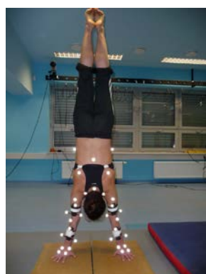
Figure 4. Handstand calibration trial and marker placement on gymnast body.
