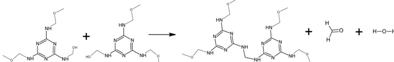
**Figure 8:** Mechanism of formaldehyde release during the polycondensation reaction of melamine-formaldehyde prepolymers
