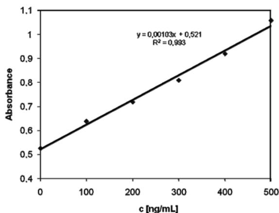
**Figure 6:** Malachite green method, lower concentration range: the absorbance of the reaction mixture 60 s after the initiation of reaction for concentrations of formaldehyde 0–500 ng/ml (0–500 ppm). Conditions: 0.37 mg/ml sulphite,  $10^{-4}$  g/ml malachite green, pH = 8, T = 24.5 °C
