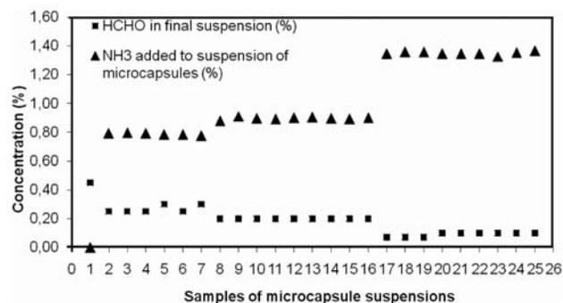
**Figure 9:** Effect of ammonia scavenger concentration on the residual formaldehyde concentration, measured in 25 batches of final microcapsule suspensions produced in a 200 l reactor
