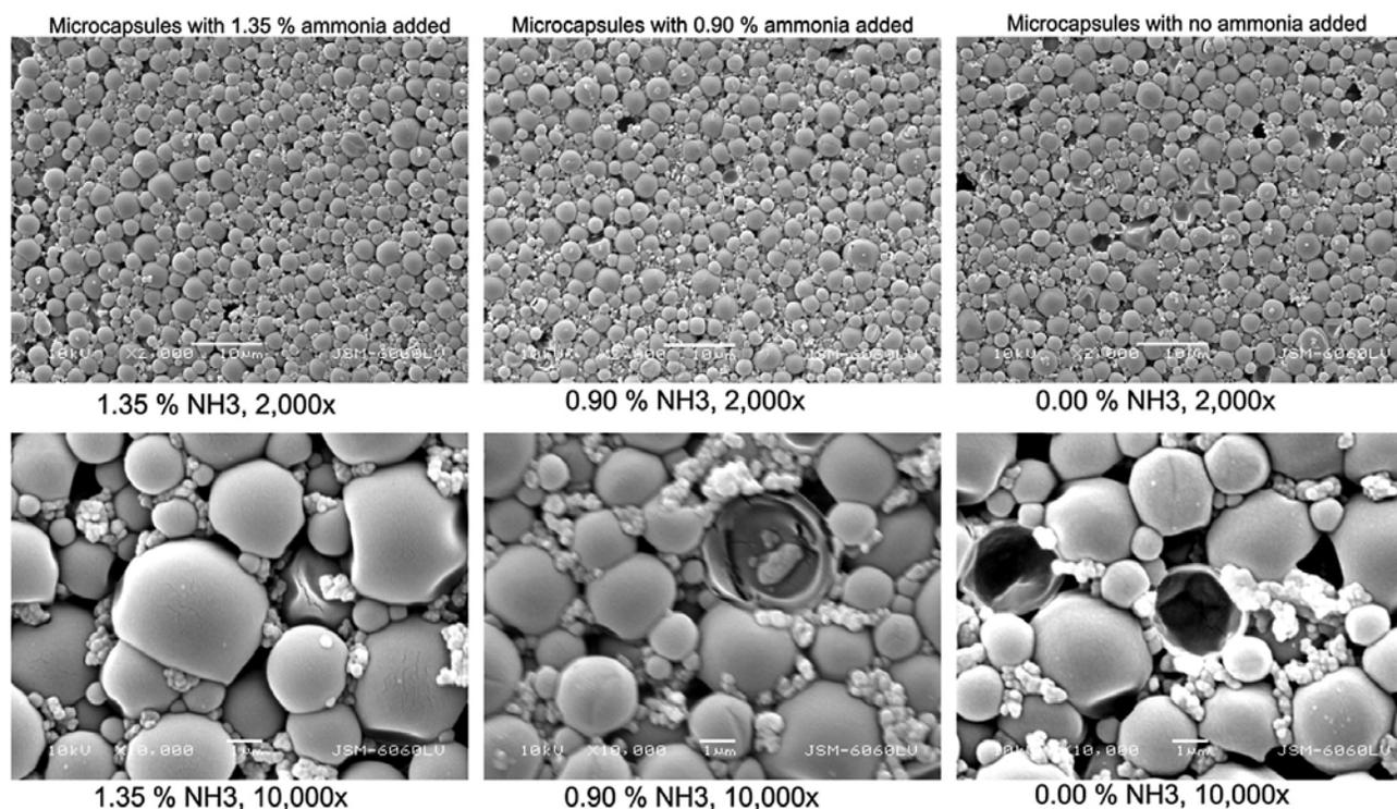
**Figure 12:** Comparison of microcapsule morphology and damage in relation to ammonia scavenger concentration (1.35%, 0.90%, 0.00%); cracking and opening of microcapsule wall appeared more frequently in a sample with no ammonia added (SEM 2000x, 10000x)
