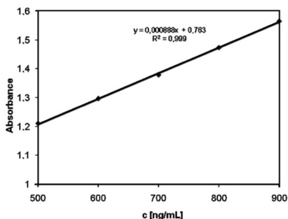
**Figure 5:** Malachite green method, higher concentration range: the absorbance of the reaction mixture 60 s after the initiation of reaction for concentrations of formaldehyde 500–900 ng/ml (0–500 ppm). Conditions: 0.37 mg/ml sulphite,  $10^{-4}$  g/ml malachite green, pH = 8, T = 24.5 °C
