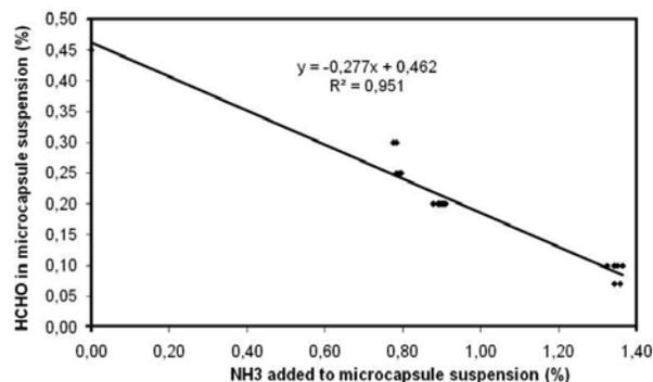
**Figure 10:** Correlation between the added ammonia scavenger concentration and the residual formaldehyde concentration; measurements from 25 batches of final microcapsule suspensions produced in a 200 l reactor
