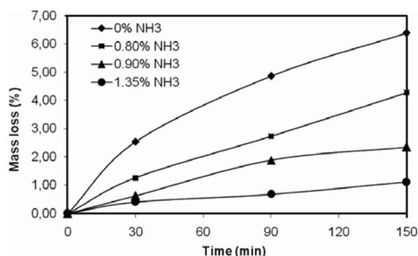
**Figure 11:** Mass loss of microcapsule samples from four different batches: with 0.00%, 0.80%, 0.90% and 1.35% ammonia scavenger in the microcapsule suspension after the polycondensation process
