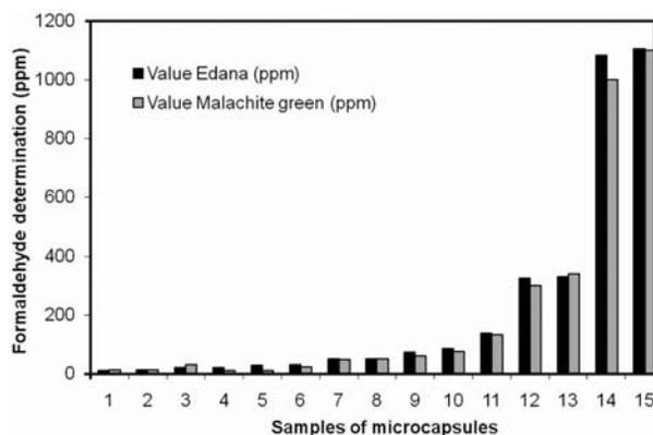
**Figure 7:** Comparison of EDANA 210.1-99 and malachite green methods: results of parallel independent analyses of 15 microcapsule samples in the formaldehyde concentration range of 10 to 1100 ppm
