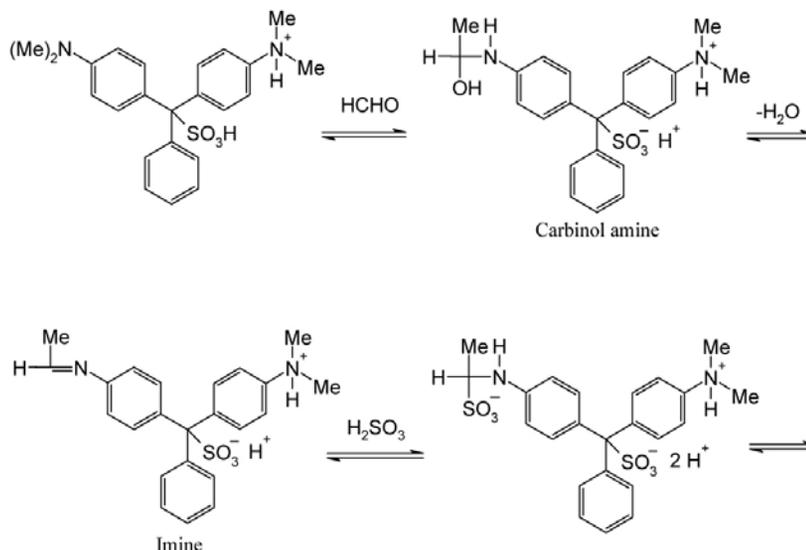
**Figure 4:** Regeneration of the chromophore system of malachite green (adaptation of a mechanism based on Keuch60)
