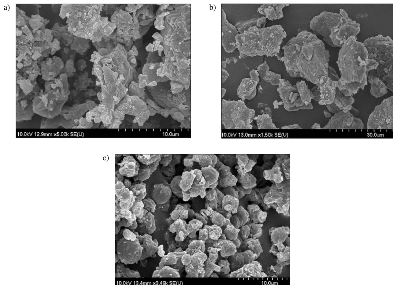
Figure 1b. Morphology by SEM of PHCl-sp (a), PHCl+M-sp (b) and PHCl-mcomp (c)
