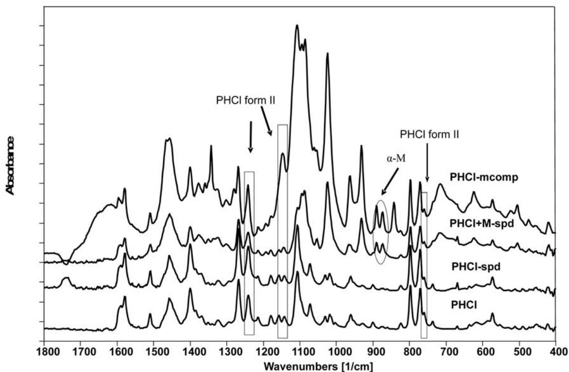
**Figure 3.** FT-IR spectra of PHCl and the samples
