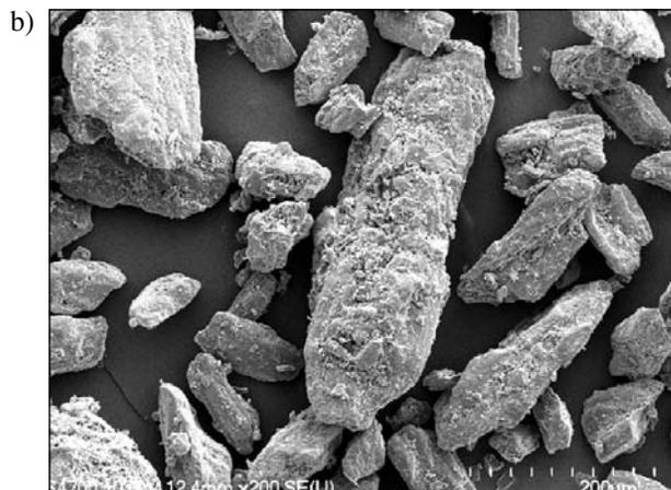
Figure 1a. SEM pictures of raw PHCl (a) and  $\beta$ -D-mannitol (b)
