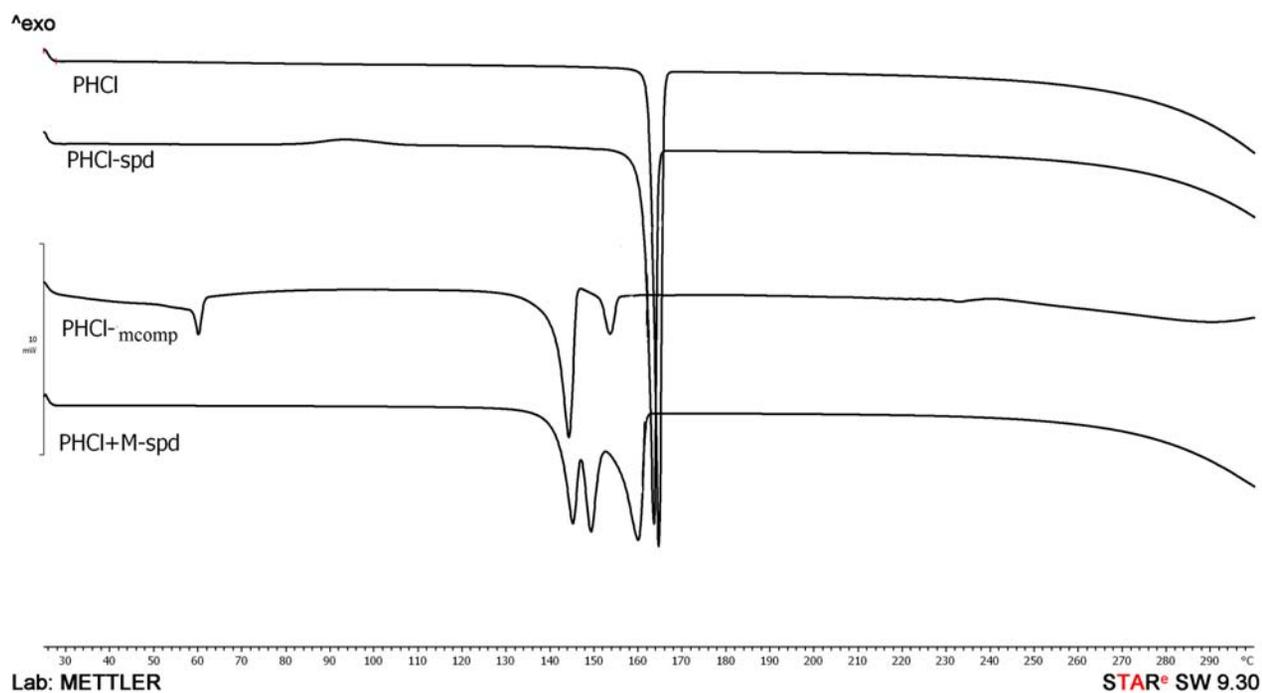
Figure 2. DSC curves of propranolol hydrochloride and the prepared samples
