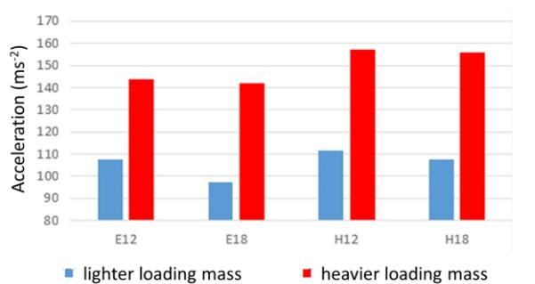
**Figure 5: The influence of the location of signal acquisition (E12, E18, H12, H18) and the weight mass on the dynamic response of the measuring plate**
