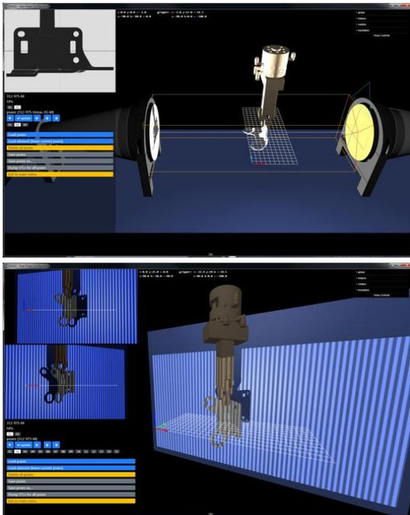
Figure 1: (up) 2D and (down) 3D measuring method
