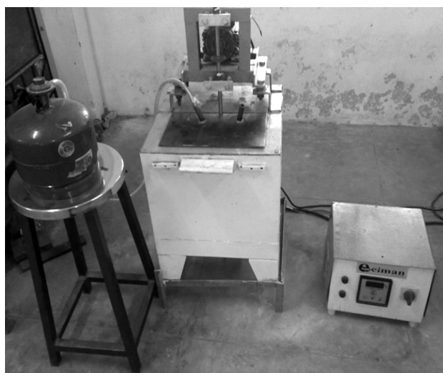
Figure 1: Two-stage stir-casting setup
