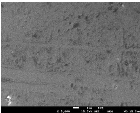
**Figure 2:** Microstructure of hardened DIN 1.7225 standard material (SEM)
