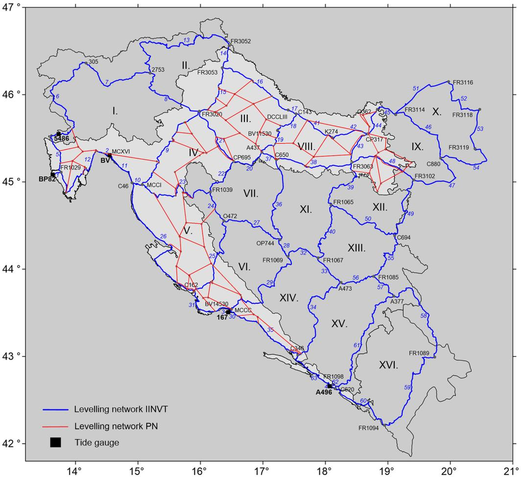
Figure 1: Configuration scheme of the IINVT and PN levelling networks on the Croatian territory
