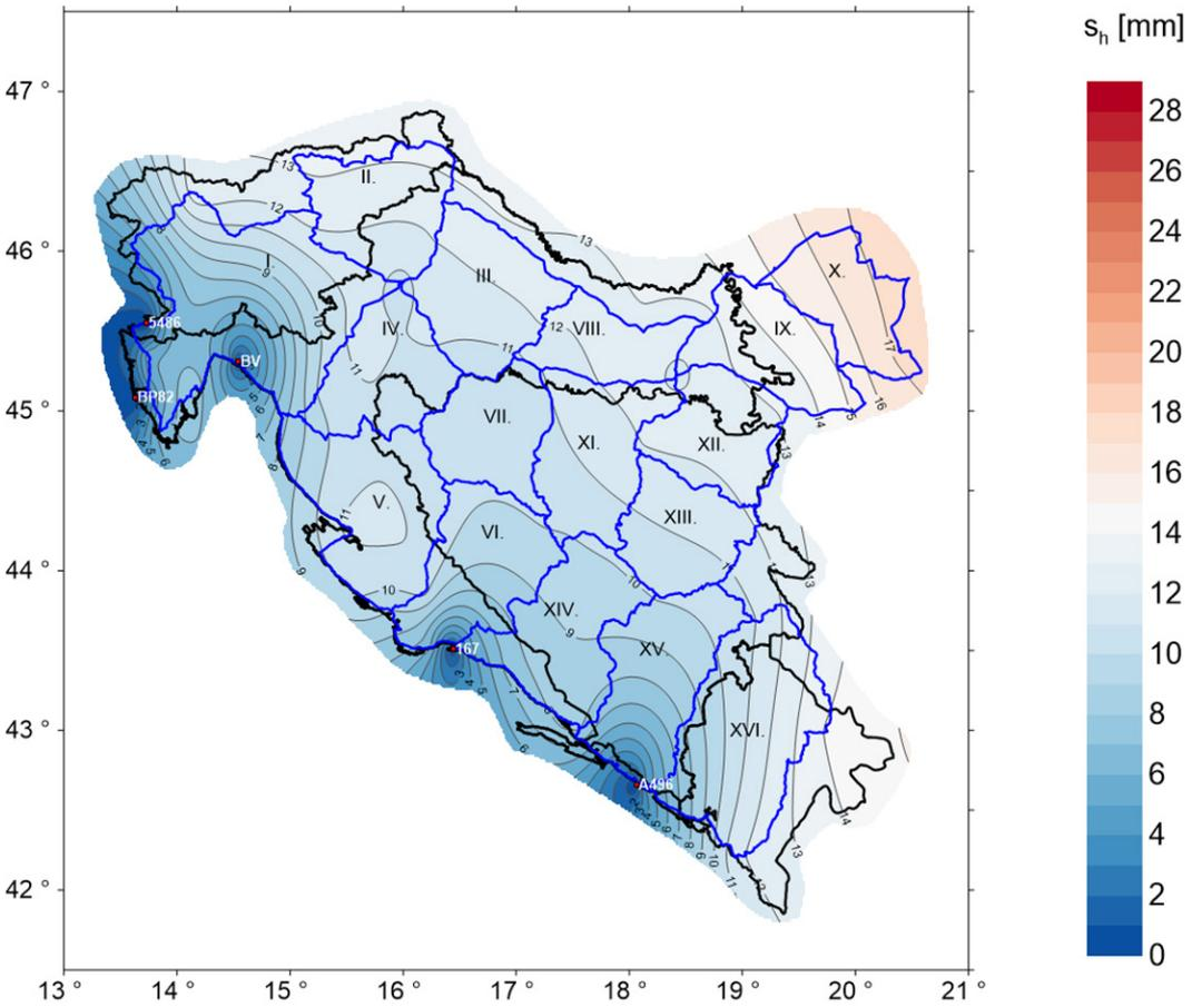
Figure 2: Height accuracy distribution of the benchmarks within the IINVT levelling network
