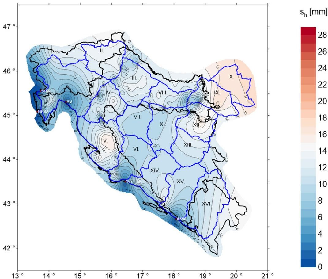
Figure 3: Height accuracy distribution of the benchmarks within the IINVT and PN levelling networks obtained from the adjustment using the hierarchical principle
