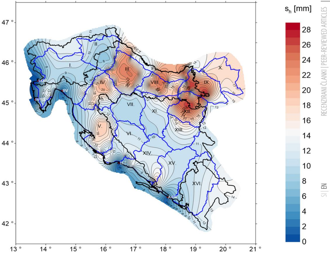
Figure 4: Height accuracy distribution of the benchmarks of the IINVT and PN levelling networks obtained from the parametric least squares adjustment of correlated measurements
