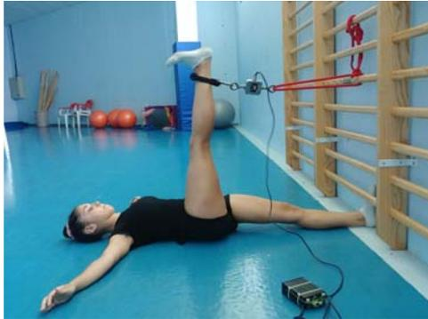
Figure 5. Maximal isometric hip flexion strength measured with a load cell.
