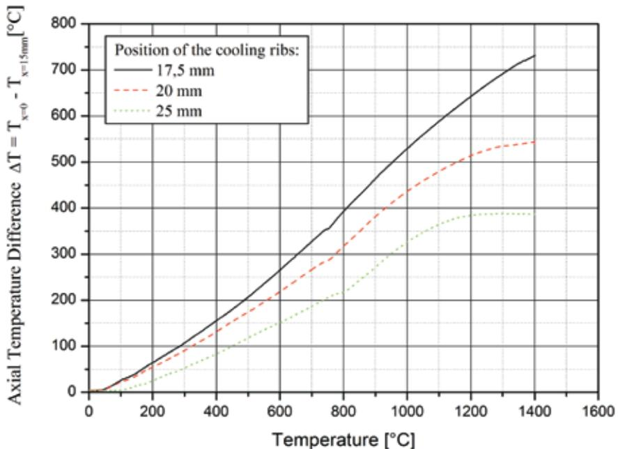
**Figure 3.** Comparison of axial temperature difference measured between the center part of the specimen and 15 mm from the center along the axis of the specimen, using different placements of the water-cooled copper ribs (17.5, 20, and 25 mm from the center of the specimen)
