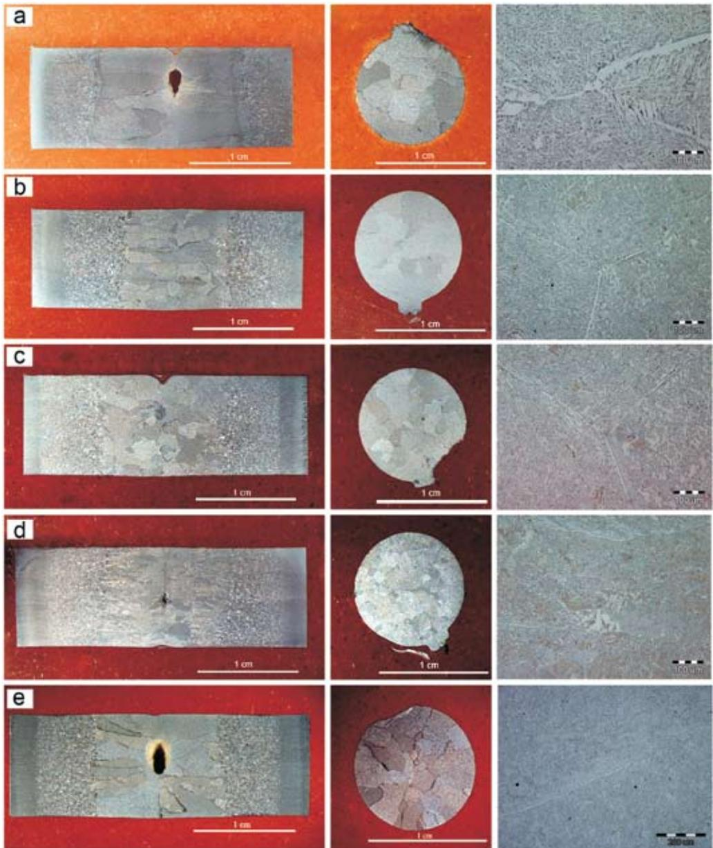
**Figure 5.** Longitudinal and axial cross-section of the isolated specimens with cooling rates 1 °C/s, 3 °C/s, 5 °C/s, 10 °C/s from a) to d) respectively and an un-isolated specimen e) with cooling rate 3 °C/s
