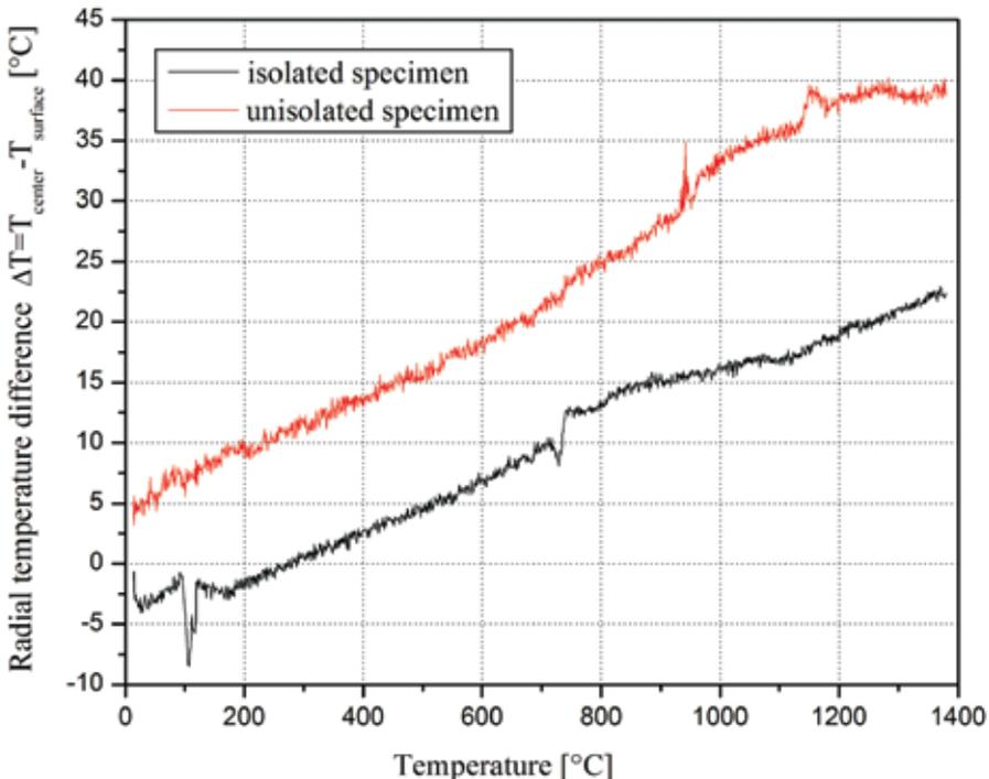
**Figure 4.** Comparison of the measured radial temperature difference between isolated and un-isolated specimens
