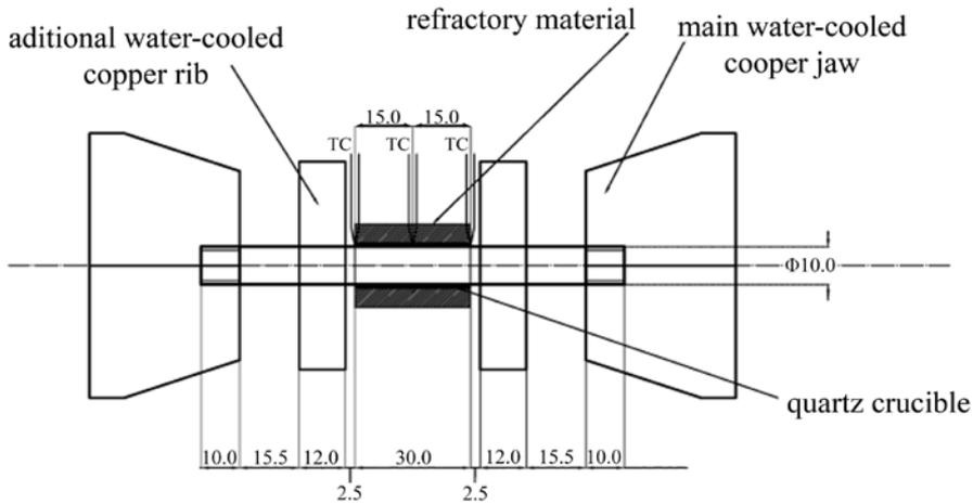
**Figure 2.** Schematic plan of the mounted specimen
