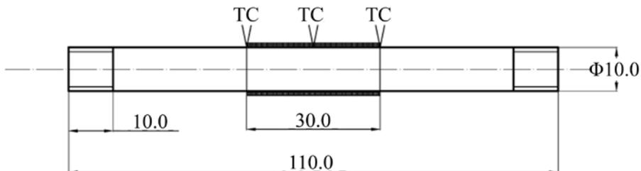
**Figure 1.** Cross section of the specimen
