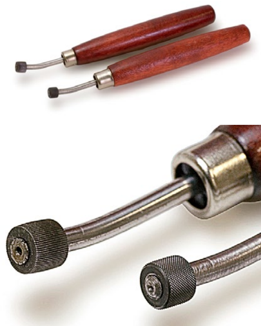
Slika 16: Roulette – orodje za rastriranje in povečava (Musashino Art University, MAU Art & Design glossary, 2024)
