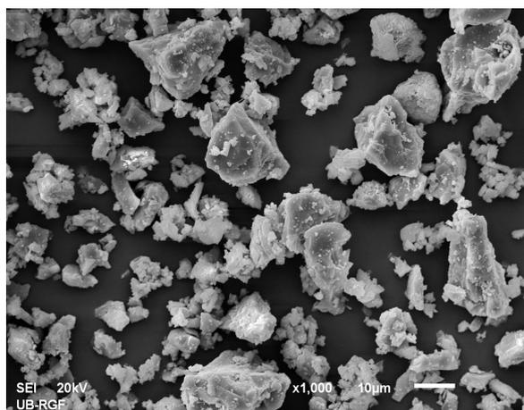
**Figure 3:** Mullite particles (SEM)
