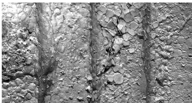
**Figure 7:** Appearance of the mullite-based lining on a test sample with visible flaws
