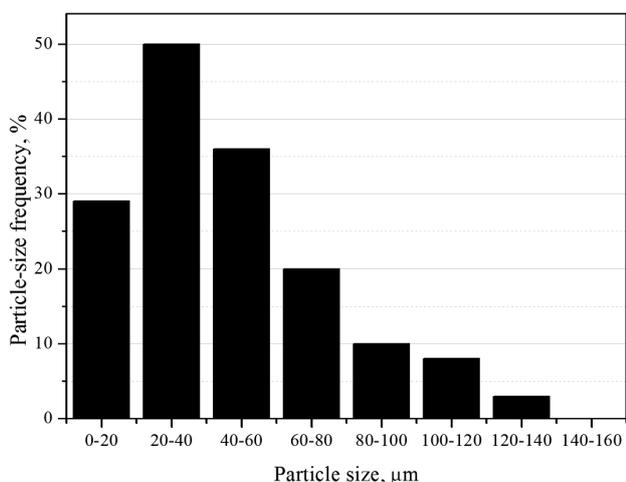
**Figure 4:** Mullite-particle size frequency
