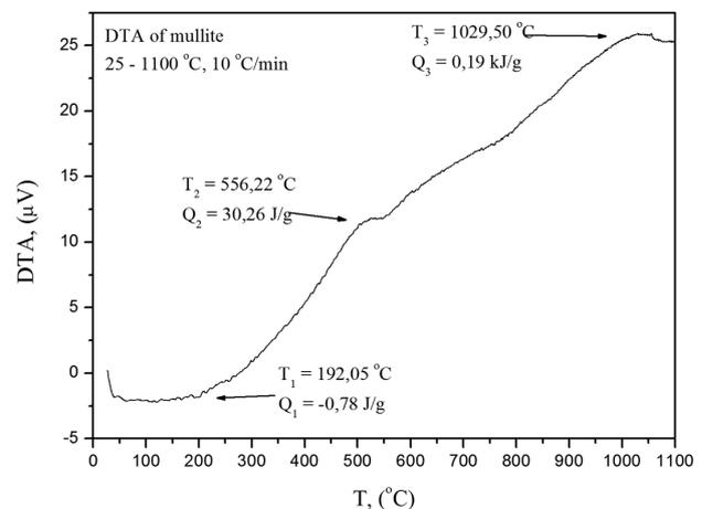
**Figure 2:** DTA curve of mullite
