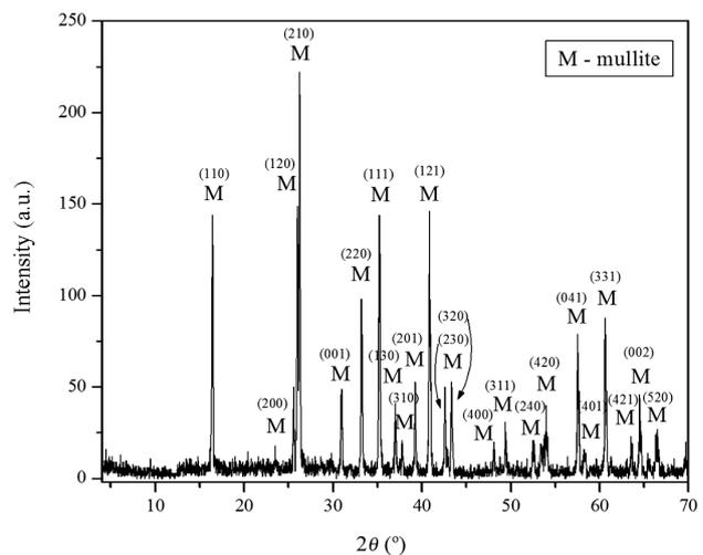
**Figure 1:** X-ray diffractogram of mullite
