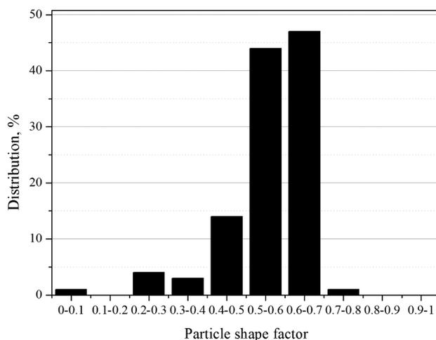
**Figure 5:** Distribution of the particle-shape factor of mullite
