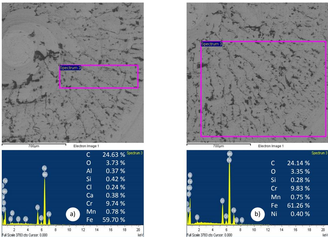
**Fig. 8** EDS analysis of emulsion-cooled specimen: a) without and b) after exposure to the electrolyte
