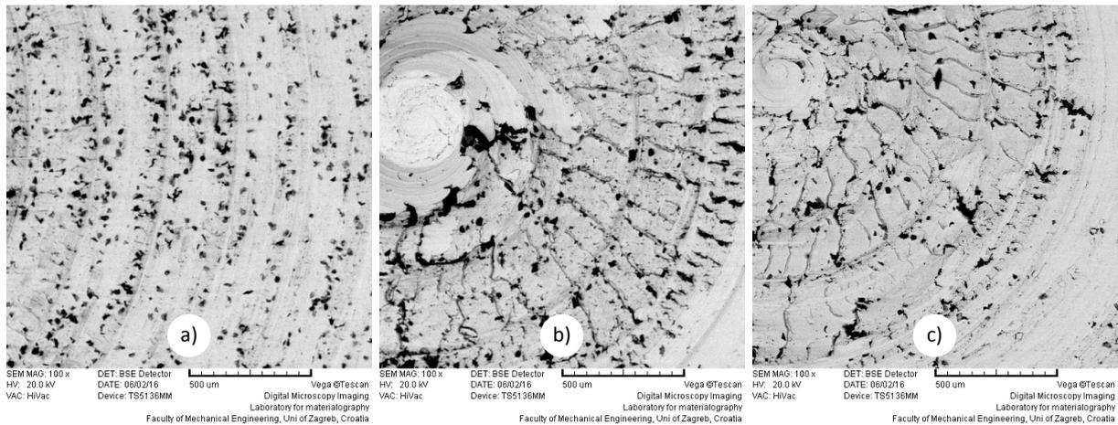
**Fig. 5** Images of surfaces for the specimens without exposure to the electrolyte: a) basic specimen, b) emulsion-cooled specimen, c) vortex tube cooled specimen
