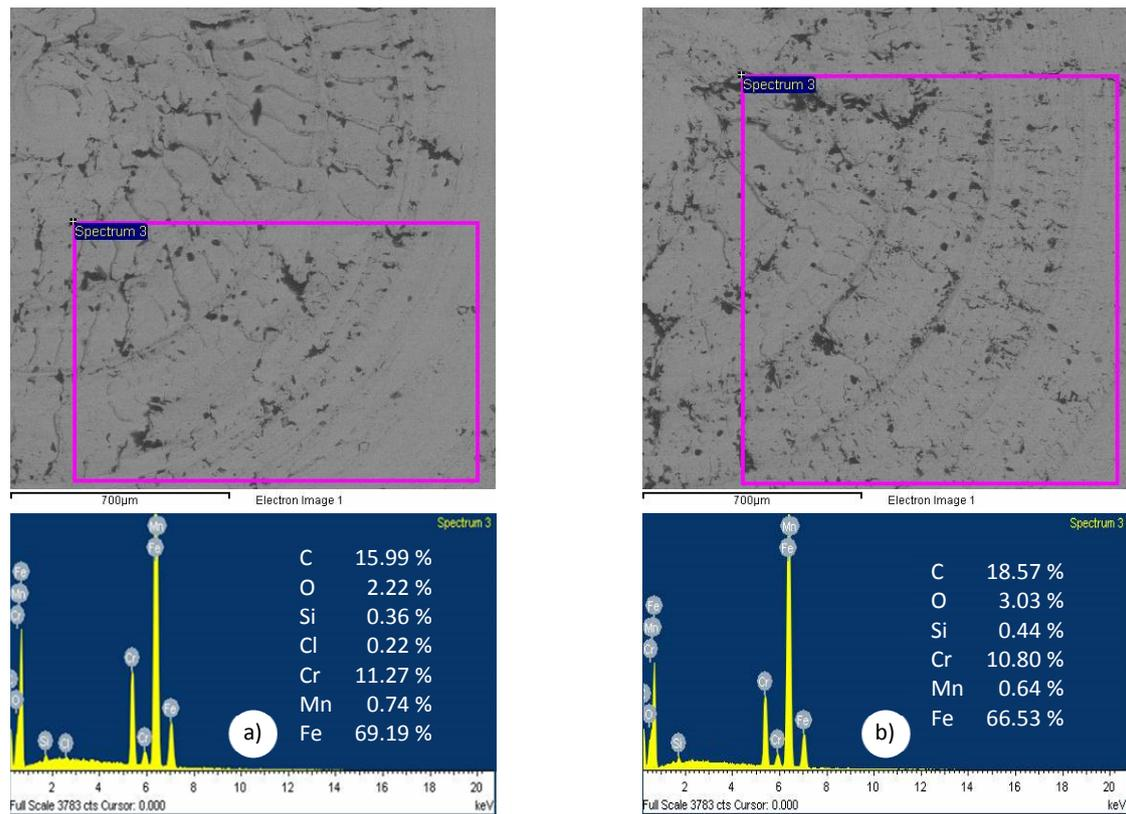
Fig. 9 EDS analysis of vortex tube cooled specimen: a) without and b) after exposure to the electrolyte
