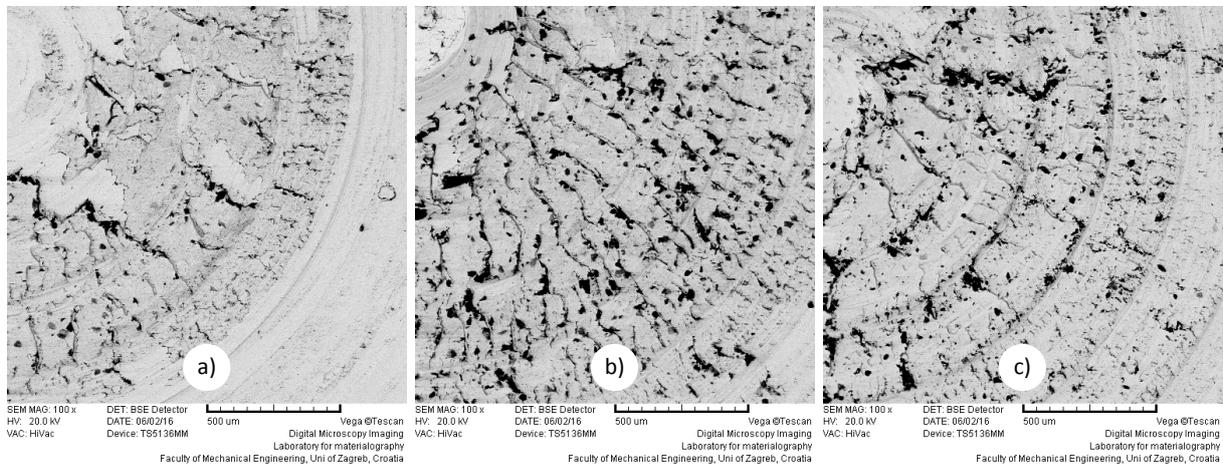
**Fig. 6** Images of surfaces for the specimens after exposure to the electrolyte: a) basic specimen, b) emulsion-cooled specimen, c) vortex tube cooled specimen
