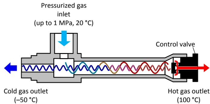
Fig. 2 Ranque-Hilsch counter-flow vortex tube – scheme of working principle
