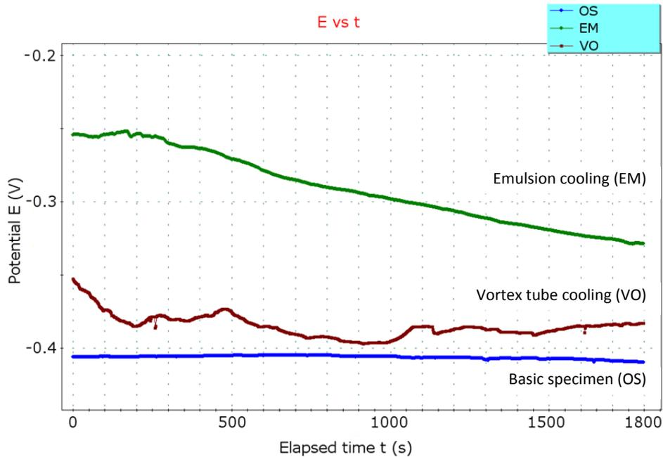
Fig. 3 Open circuit potential vs. time of exposure for specimens in 3.5 % aqueous solution of NaCl
