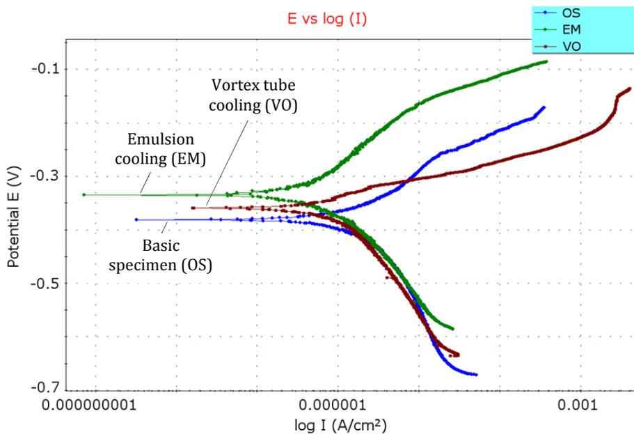
Fig. 4 Polarization behaviour for specimens in 3.5 % aqueous solution of NaCl
