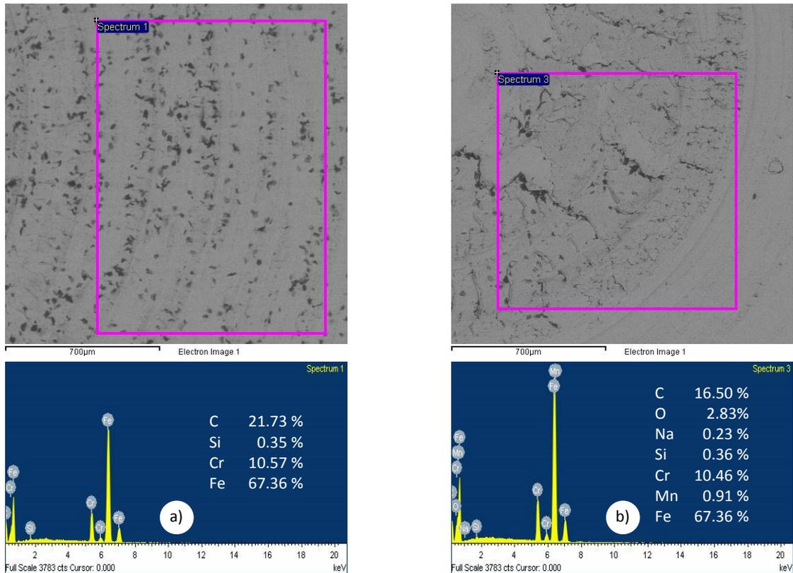
**Fig. 7** EDS analysis of basic specimen: a) without and b) after exposure to the electrolyte
