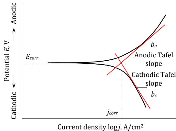
Fig. 1 A schematic illustration of the Tafel extrapolation method
