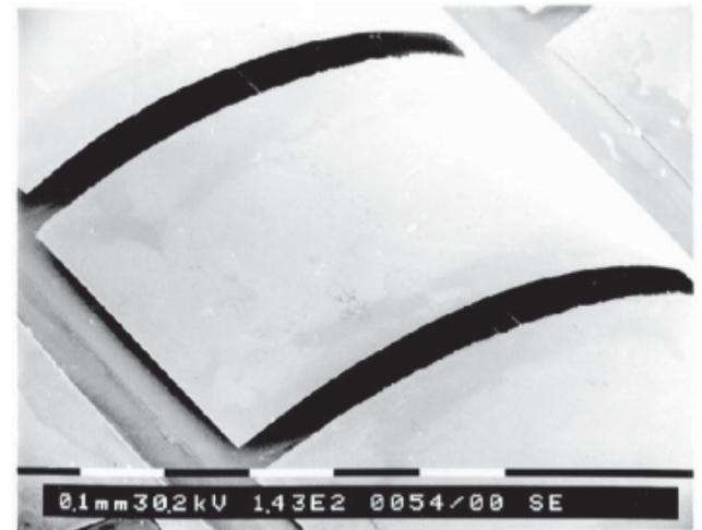
Fig.6. Examples of stress induced microfabrication, microcoils and flexible elements for electrostatic actuators
