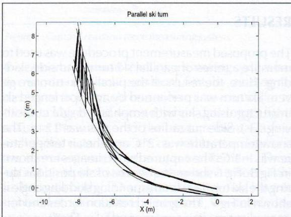
Figure 6. Measured ski turn (top view). Plotted trajectories connect marker position. Skis position is outlined for each third measured position.
