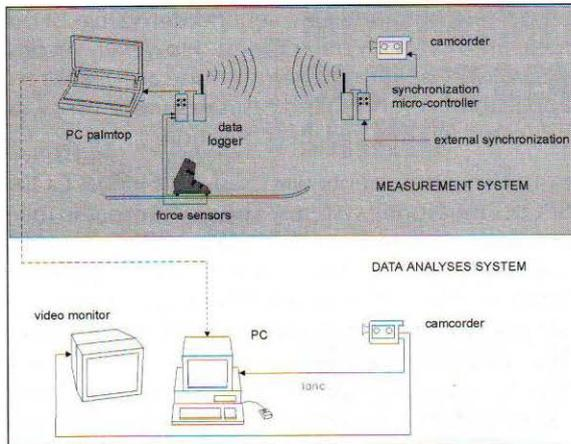
Figure 1. Ground reaction force measuring system
