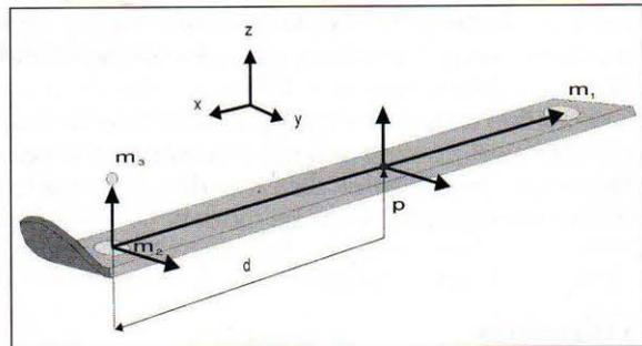
Figure 3. Marker placement and notation
