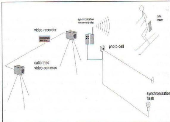
Figure 2. Synchronisation scheme of kinematic measuring system and ground reaction measuring system
