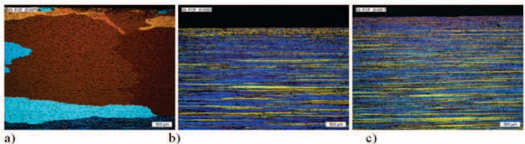
**Figure 5.** Polarized light micrographs of the extruded rods in longitudinal section a) process K, b) process PQ and c) process BQ (4 s)
