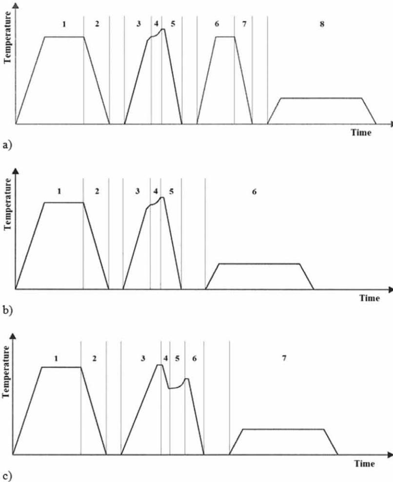
**Figure 1.** Scheme of the extrusion processes a) conventional, K (1-homogenization, 2-cooling, 3-reheating, 4-extrusion, 5-cooling, 6-solution treatment, 7-quenching and 8-artificial aging), b) press-quenching, PQ (1-homogenization, 2-cooling, 3-reheating, 4-extrusion, 5-quenching and 6-artificial aging) and c) billet-quenching, BQ (1-homogenization, 2-cooling, 3-preheating above the solvus temperature, 4-cooling to the forming temperature, 5-extrusion, 6-quenching and 7-artificial aging)
