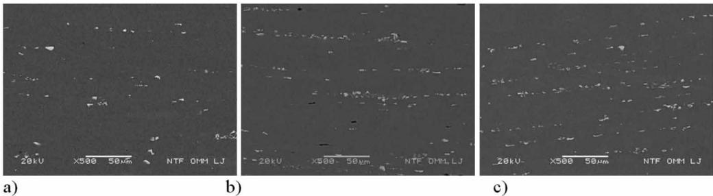
**Figure 4.** Back scattered electron micrographs of the extruded rods in longitudinal section from billets that were homogenized at the temperature of 480 °C/5 h a) process K, b) process PQ and c) process BQ (4 s)
