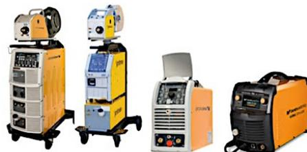
**Varmig 271-i LCD** (MAG, MIG, FCAW, SMAW); **VARTIG 221 AC/DC** (TIG, SMAW); **VPS 4000** (MAG, MIG, FCAW SMAW); **Welbee 500L** (MAG, MIG, FCAW, SMAW) **Daihen Varstroj**; **AVP A13**, **Rade Končar 1000 A** (EPP) **AVP**; **Flame Welding & Cutting Kit Messer**. The equipment enables the production of welded joints using REO, MAG, MIG, TIG, EPP, FCAW procedures, as well as cutting of the base material and welds.
