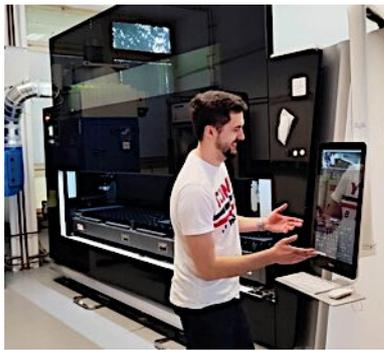
**CNC laser sheet metal cutting machine Bodor i7 Bodor**
