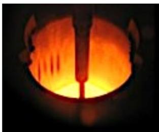
Melting in a vacuum induction furnace
