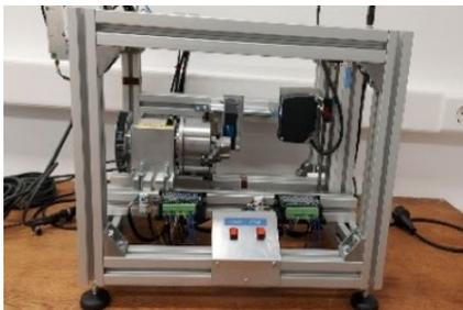
**Laser measuring cell SICK FS, LAMEH**
