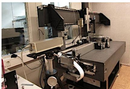
**2D measuring device with sub-micrometre resolution**
