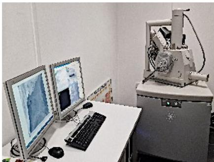
**QUANTA 200 3D Electron Ray Microscope with focused ion beam (SEM/FIB) FEI Company**
