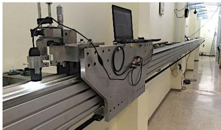
**Measuring stage 13M LTM UM FS LTM in-house production.** We use the measuring stage of our own production for the calibration of industrial line scales and tape measures. The device has a measuring range of 12 m, but by folding the gauge, we can also calibrate tape measures up to 200 m. The device is equipped with a magnetic measuring encoder with a resolution of 1  $\mu\text{m}$ , and a laser interferometer can also be integrated into the device for very precise measurements.
