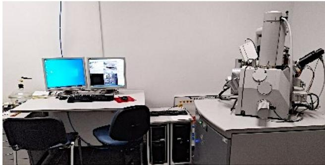
**The QUANTA 200 FEI 3D Environmental Line Electron Microscope with an Ion Gun and Platinum Deposition System** is an environmental electron microscope with thermal emission of electrons. The microscope allows you to work at different pressures and at 100% humidity. The environmental mode of operation – ESEM, is suitable for the analysis and characterisation of non-conductive samples (polymeric materials, ceramics, non-conductive surface layers, biological and medical preparations, etc.), and is
