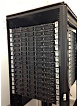
**HPC CORE@UM** is a micro supercomputer with 3 TERAFLIPS of computing capacity, designed to perform complex scientific computer simulations. The installed software enables the implementation of complex nonlinear simulations of the behaviour of solids and liquids and multiphysical problems for a wide range of research and industrial applications.
