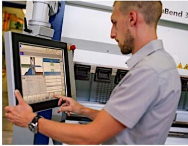
**CNC sheet metal bending machine TruBend 3066 Trumpf**
