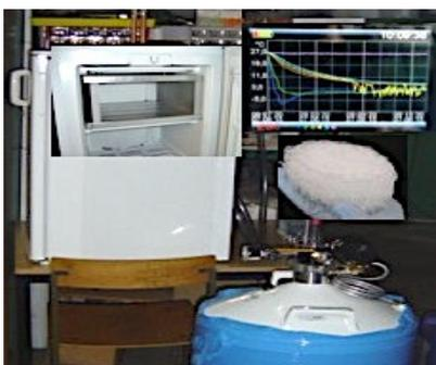
**Chamber for one-sided freezing of liquid samples (porosity gradient) LBBE FS**
