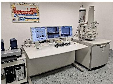
**HRSEM electron scanning microscope SIRION 400 FEI Company, equipped with an EDS analyser for microchemical analyses INCA 350 Oxford Instruments**
