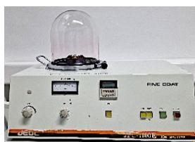
**Jeol JFC 1100E Thin Metal Coating Sprayer Jeol**
