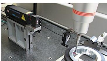
**Laser Interferometer LSP 30 Lasertex Poland**
