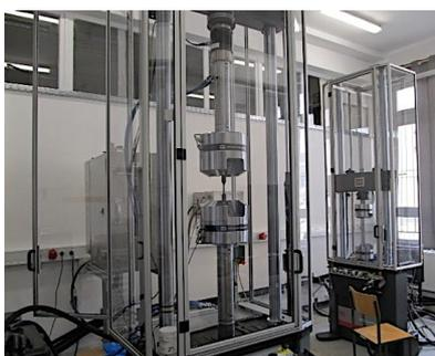
**MTS servo-hydraulic machines for single-axis and two-axis testing MTS System USA**
