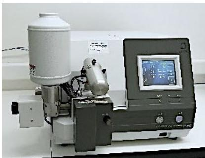
**COOLING CROSS SECTION POLISHER IB-19520CCP JEOL**
