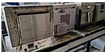
**Furnaces for alloy smelting and heat treatment Bosio**
