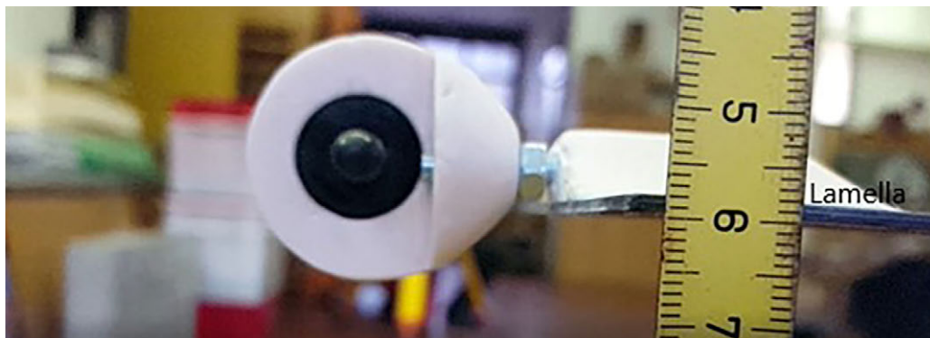
Figure 6: The setting of the prism and measuring tape at the end of the lamella (Source: own) .
