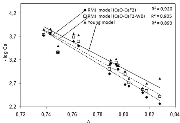
Figure 2: Sulphide capacity as the function of optical basicity
