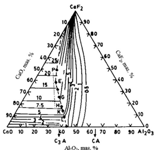
Figure 1: Sulphide capacity for the CaO-CaF<sub>2</sub>-Al<sub>2</sub>O<sub>3</sub> system at 1500 °C
