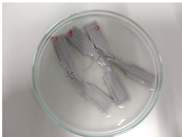
Fig. 3. Samples after 3 hours of liquid acetone treatment
