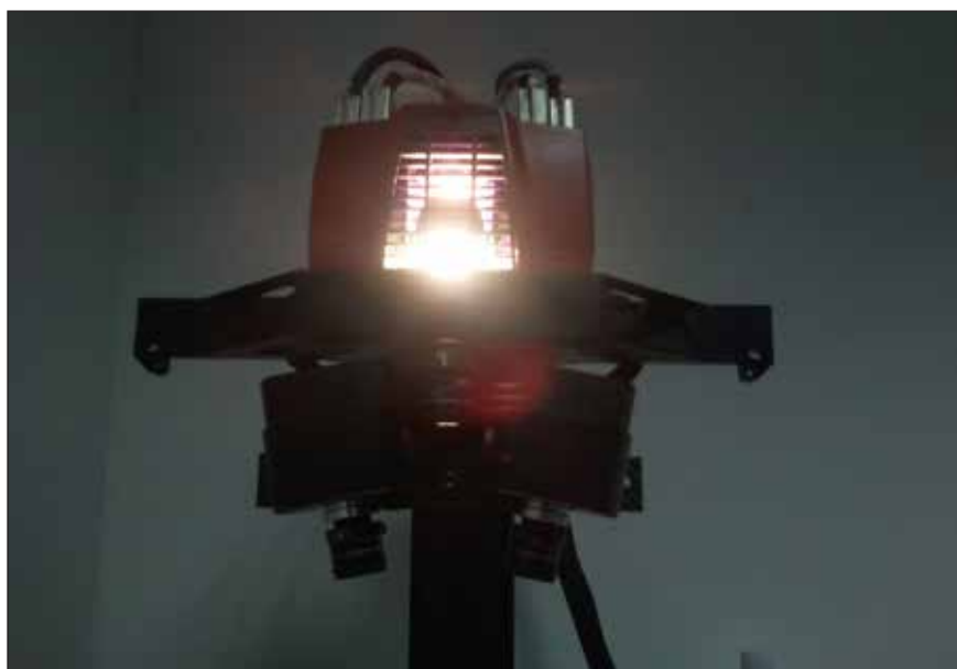
Figure 3. Optical 3D digitizer ATOS II SO with two high-resolution CCD cameras
