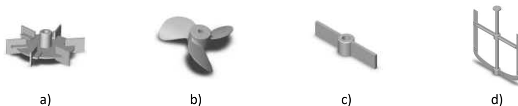
Slika 5.1: Različni tipi mešal: a) Rushtonova turbina, b) propeler, c) veslo, d) sidro ( http://www.postmixing.com/mixing%20forum/impellers/rt.htm )
