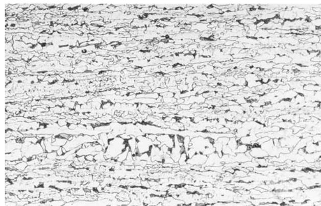
**Figure 5:** (magn. 200 times) Microstructure of the steel K from **Figure 3** rolled in the temperature range from 900 °C to 774 °C
