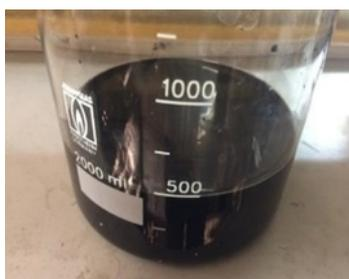
**Fig. 2.** The nanofluid sample which was prepared by using 0.2 wt.% nanoporous graphene, 0.2 wt.% CMC and DI water labelled as NPG-0.2
