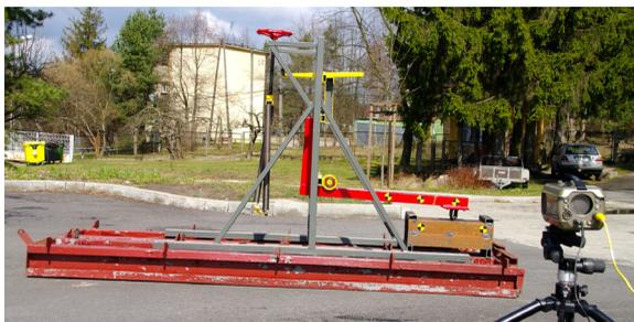
Fig. 3. The setup for performing impact energy absorption tests
