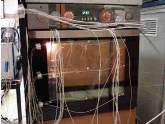
Fig. 6. Temperature measurement locations at oven outer wall and infrared heater
