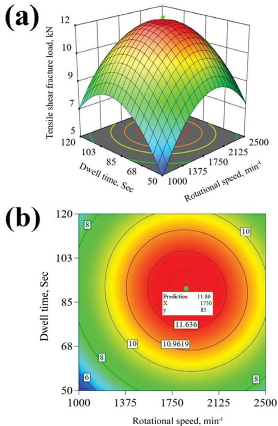
Figure 5: TSFL of FMB: a) response graph and b) contour graph
