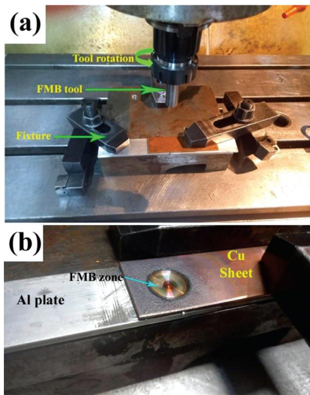
**Figure 1:** Experimental set-up with: a) tool rotational direction and fixture design and b) FMB processed sample
