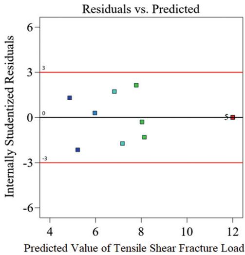
Figure 2: Internally studentized residual values for the predicted values of TSFL of FMB
