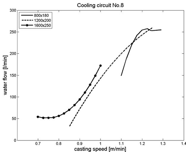
**Figure 7:** Optimal cooling curves for cooling circuit No. 8
