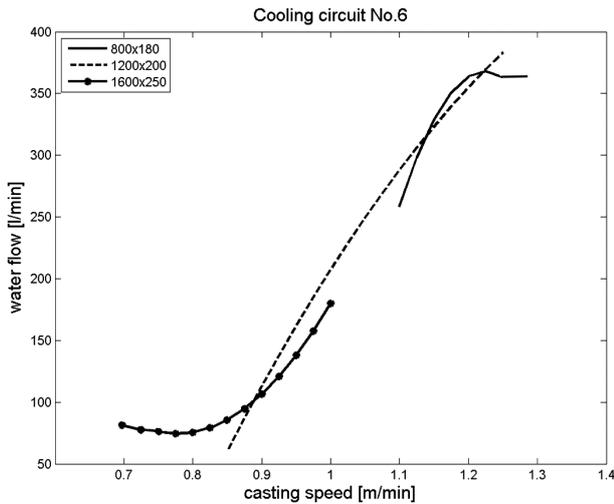
**Figure 6:** Optimal cooling curves for cooling circuit No. 6
