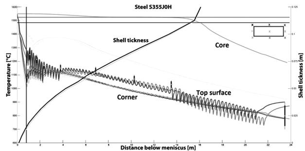
**Figure 2:** Temperatures distribution after fuzzy regulation
