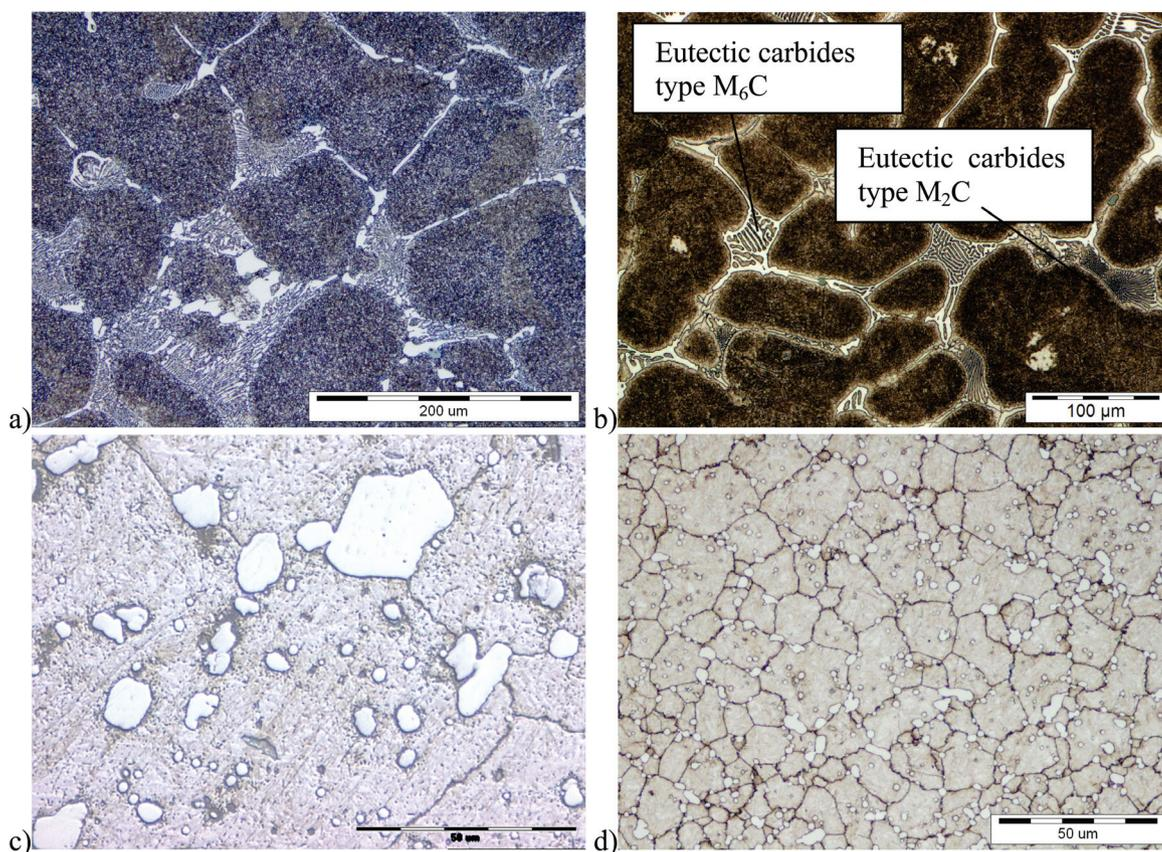
**Figure 2:** Microstructure for M42 tool steel obtained at solidification rate of 0.25 K/s (a) and at solidification rate of 0.16 K/s (b), obtained microstructure after hot rolling applying of inappropriate (too high) soaking temperature of 1 180 °C for (c) and microstructure obtained in rolled piece at appropriate soaking temperature 1 150 °C (d).
