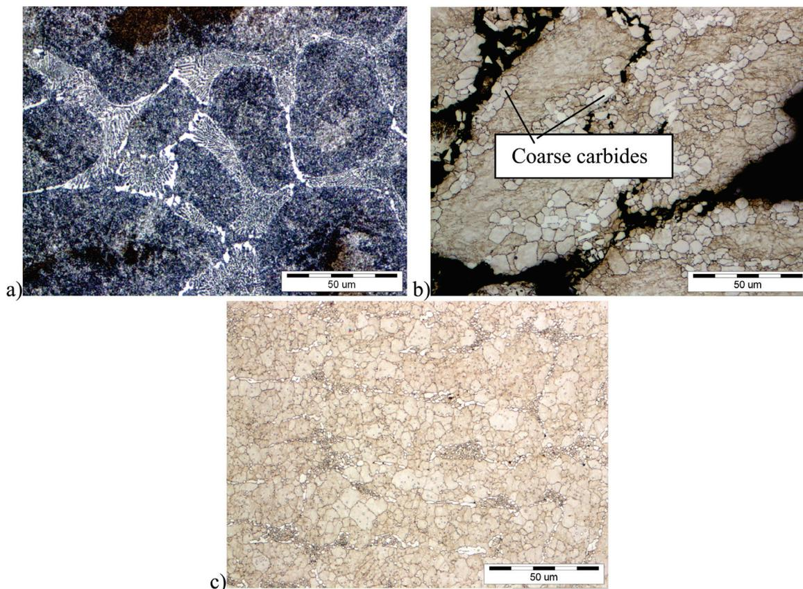
**Figure 3:** Influence of soaking temperature on coarsening of carbides and on hot deformability for continuously cast M42 tool steel on upper limit of temperature range: initial as-cast microstructure (a); soaking and deformation temperature 1 170 °C (b); soaking and deformation at temperature of 1 140 °C (c).
