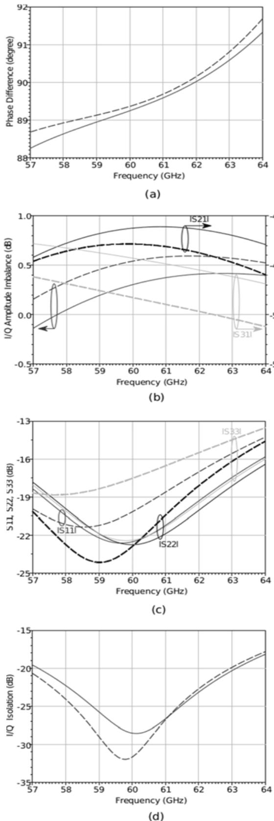
**Figure 8:** The performance of differential branch-line coupler: (a) phase difference, (b) insertion loss, (c) reflection coefficient, (d) isolation.
