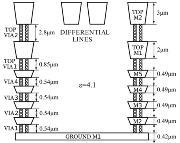
**Figure 6:** Technology metal stack.
