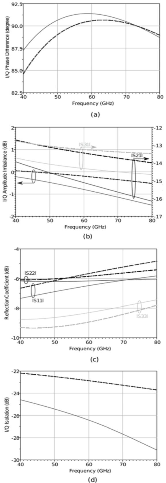
**Figure 12:** The performance of the 60 GHz poly-phase filter: (a) phase difference, (b) insertion loss, (c) reflection coefficient, (d) isolation.
