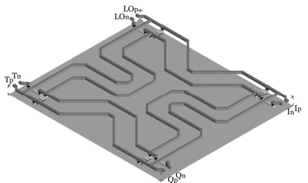
**Figure 7:** 3D preview of the differential branch-line coupler.
