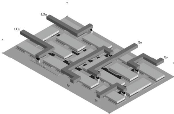
**Figure 11:** 3D preview of the 60 GHz poly-phase filter.
