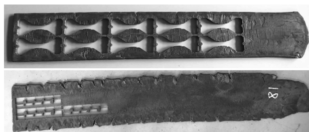
Figure 4: Positions of specimens on a rolled semi-product: a) type 1, b) type 2
