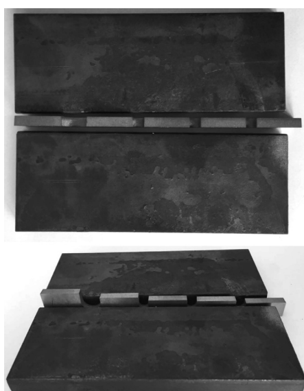
Figure 3: Positions of specimens between holding plates
