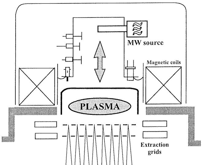
Figure 16: ECR ion beam source
