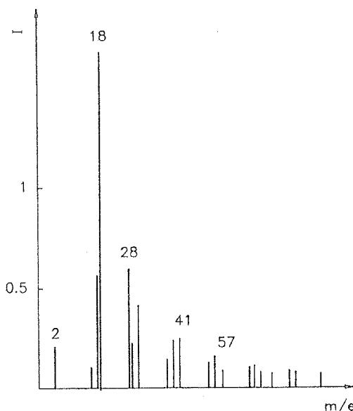
Fig. 5: Mass spectrum of the outgassing products from the electrochemically gold plated (citrate electrolyte) contact alloy Argelec 181 ( $135^{\circ}\text{C}$ ,  $1\times 10^{-6}$  mbar) after 24 hours of outgassing.
