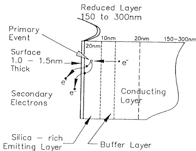
Fig. 1: Microchannel wall cross-section
