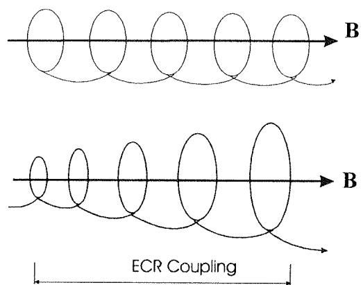
Figure 9: *Electron motion in a static magnetic field*
