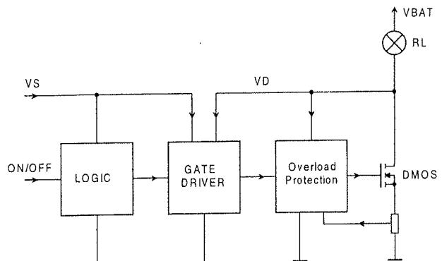
Fig. 3: Block diagram of the lamp driver circuit
