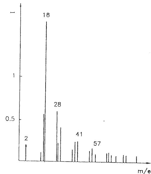
Fig. 6: Mass spectrum of the outgassing products from the electrochemically gold plated (phosphate electrolyte) contact alloy Argelec 181 ( $135^{\circ}\text{C}$ ,  $1\times 10^{-6}$  mbar) after 24 hours of outgassing.
