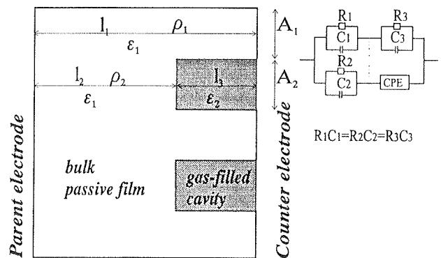
Fig. 4: Schematics of a model taking into account the poor contact at the passive film/counter electrode interface and/or film porosity.
