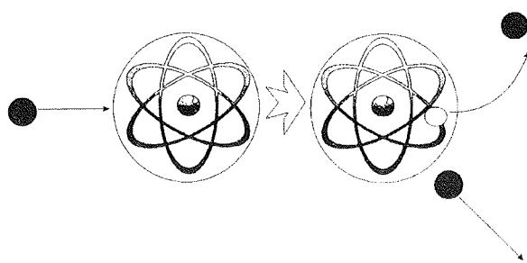
Figure 5: electron - atom inelastic collision causing ionization
