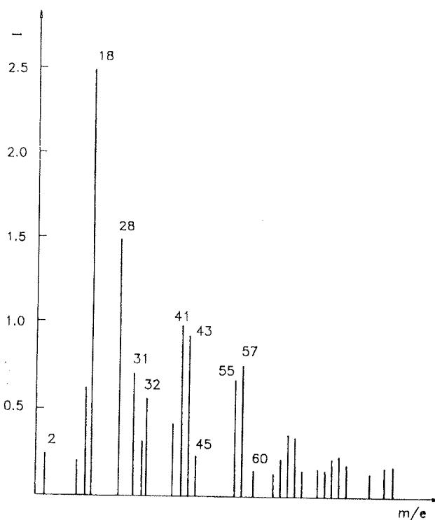
Fig. 4: Mass spectrum of the outgassing products from the electrochemically gold plated (citrate and phosphate electrolyte) contact alloy Argelec 181 (135°C,  $1 \times 10^{-6}$  mbar) after 30 minutes of outgassing.
