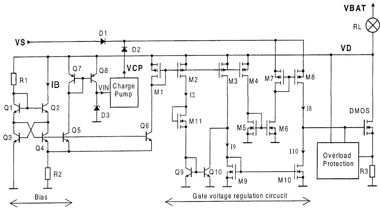
Fig. 4: Circuit diagram of the lamp driver circuit
