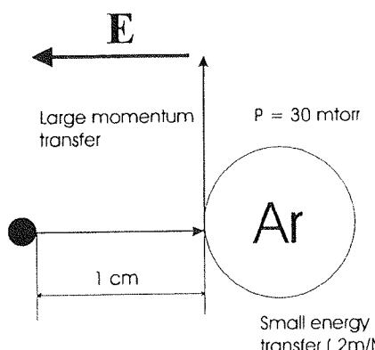
Figure 8: Elastic collision between electron and Ar atom
