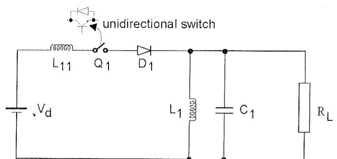
Fig. 1: The "half-wave" resonant link converter configuration
