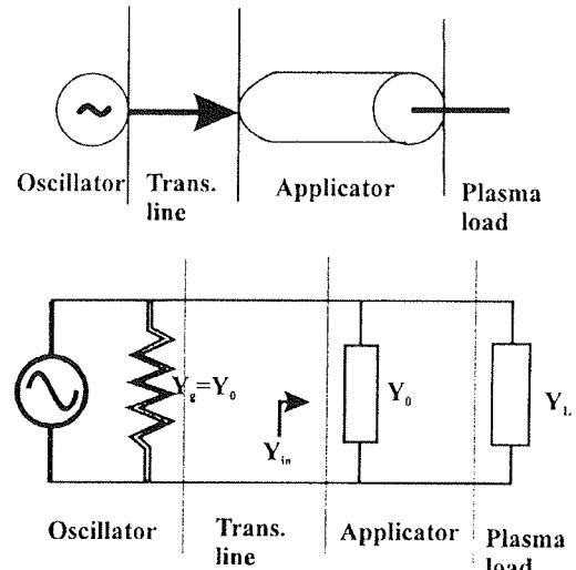
Figure 13: MW processing system and its equivalent circuit
