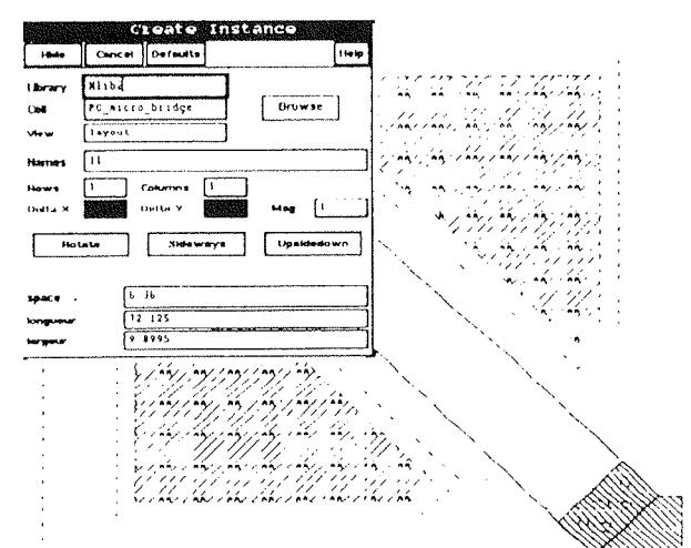
Fig. 5: Instantiation of a microbridge parametrized cell
