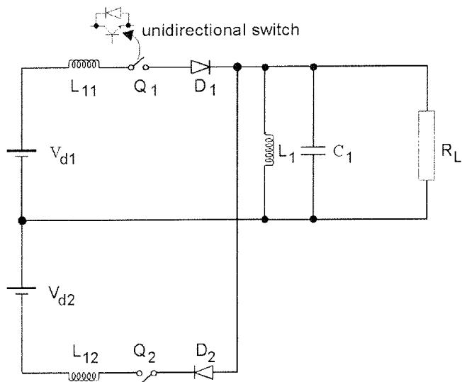
Fig. 2: The "full-wave" resonant link converter configuration
