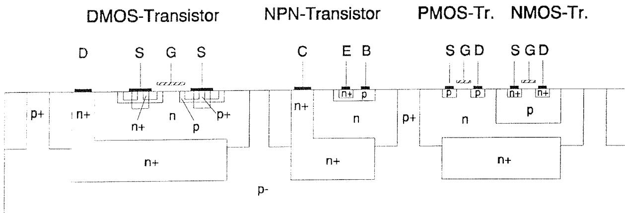
Fig. 1: Cross section of the Smart Power Technology
