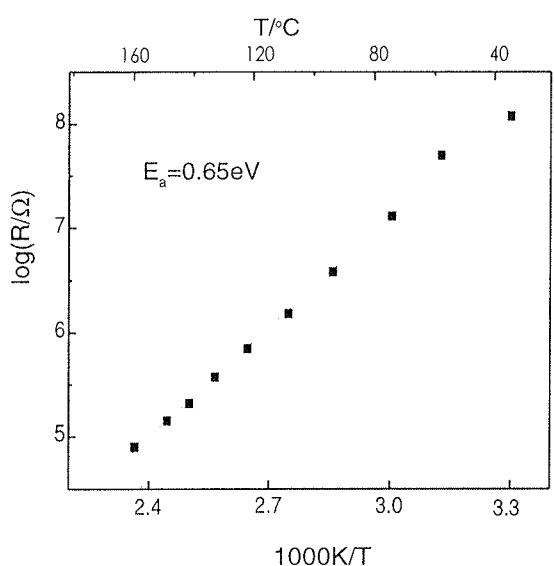
Fig. 7: Arrhenius plot showing temperature dependence of passive film conductivity.
