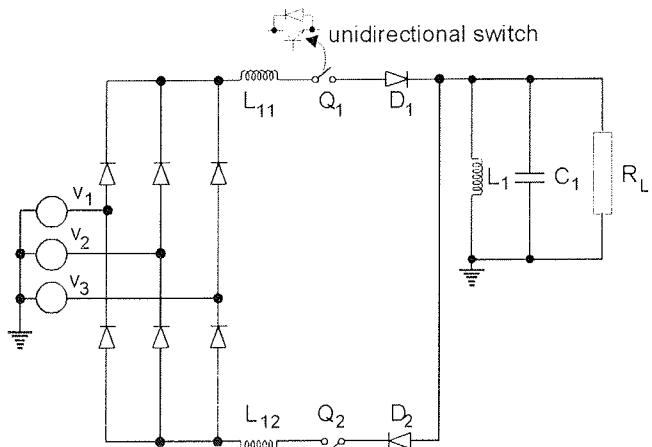
Fig. 3: The AC to HF-AC resonant link converter configuration
