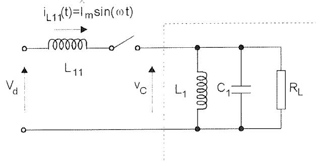
Fig. 6: The equivalent circuit for injected-absorbed current method
