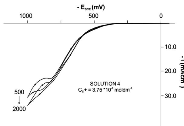
**Figure 4.** Voltammograms of cathodic polarization with  $Tl^+$ ;  $T = 343$  K, polarization rate  $20 \text{ mVs}^{-1}$ , rotation speed 500 to  $2000 \text{ min}^{-1}$ .
