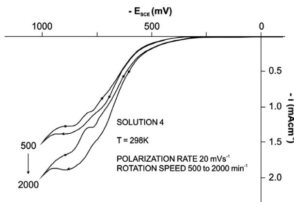
**Figure 3.** Voltammograms of cathodic polarization with  $Tl^+$ ;  $T = 298$  K, polarization rate  $20 \text{ mVs}^{-1}$ , rotation speed 500 and  $2000 \text{ min}^{-1}$ .
