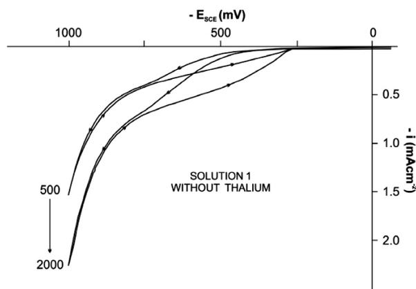
**Figure 1.** Voltammograms of cathodic polarization without  $Tl^+$ ;  $T = 298$  K, polarization rate  $20 \text{ mVs}^{-1}$ , rotation speed 500 to  $2000 \text{ min}^{-1}$ .
