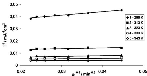
Figure 9. Dependence of  $i^{-1}$  on  $\omega^{-0.5}$  given for different temperatures  $C_{\text{Ti}^+} = 3.75 \times 10^{-5} \text{ mol dm}^{-3}$ ,  $E = 900 \text{ mV}_{\text{SCE}}$ .
