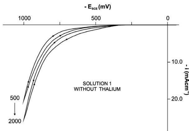
**Figure 2.** Voltammograms of cathodic polarization without  $Tl^+$ ;  $T = 343$  K, polarization rate  $20 \text{ mVs}^{-1}$ , rotation speed 500 to  $2000 \text{ min}^{-1}$ .
