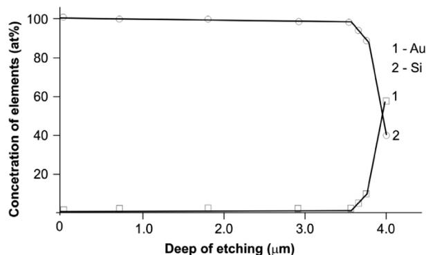
**Figure 6.** AES profile analysis of deposit;  $C_{Tl} = 3.75 \cdot 10^{-4}\text{ mol dm}^{-3}$ ,  $T = 343\text{ K}$ ,  $i = 9.87\text{ mA cm}^{-2}$ , rotation speed  $500\text{ min}^{-1}$ .
