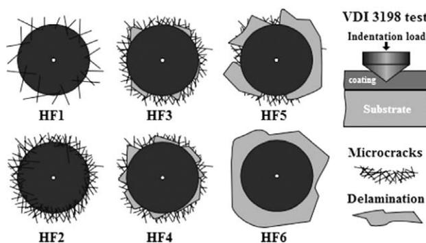
**Figure 11:** Principle of the VDI 3198 indentation test<sup>32</sup>
