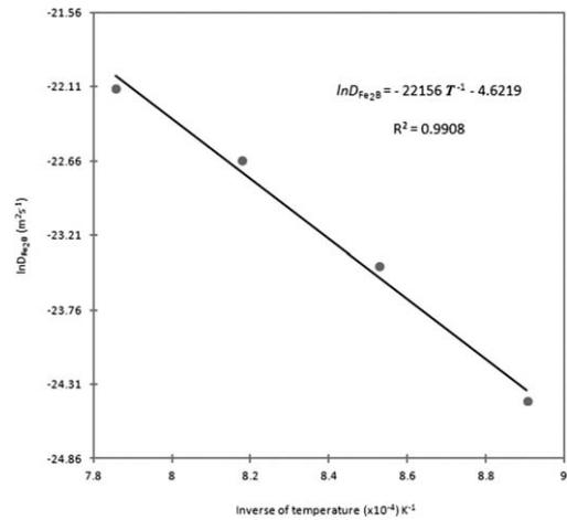
**Figure 14:** Boron diffusion coefficient ( $D_{Fe_2B}$ ) as a function of the boriding temperature
