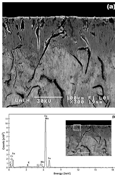
**Figure 9:** a) Micrograph image of the microstructure of the gray-cast-iron boride layer obtained at 1123 K after an exposure time of 6 h, b) EDS spectrum of a borided sample
