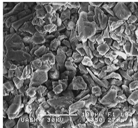
**Figure 6:** SEM image of boriding powder (B<sub>4</sub>C + KBF<sub>4</sub> + SiC)
