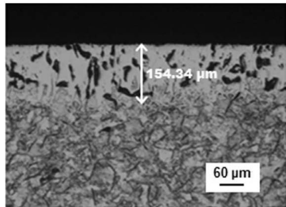
**Figure 15:** Light micrograph of the boride layer formed on gray cast iron during the powder-pack boriding at 1253 K after an exposure time of 5 h
