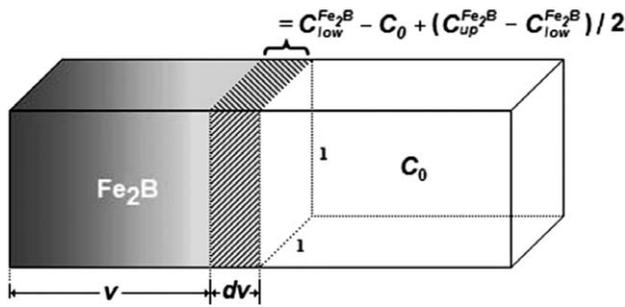
**Figure 2:** Schematic representation of the mass-balance equation at the (Fe<sub>2</sub>B/substrate) interface
