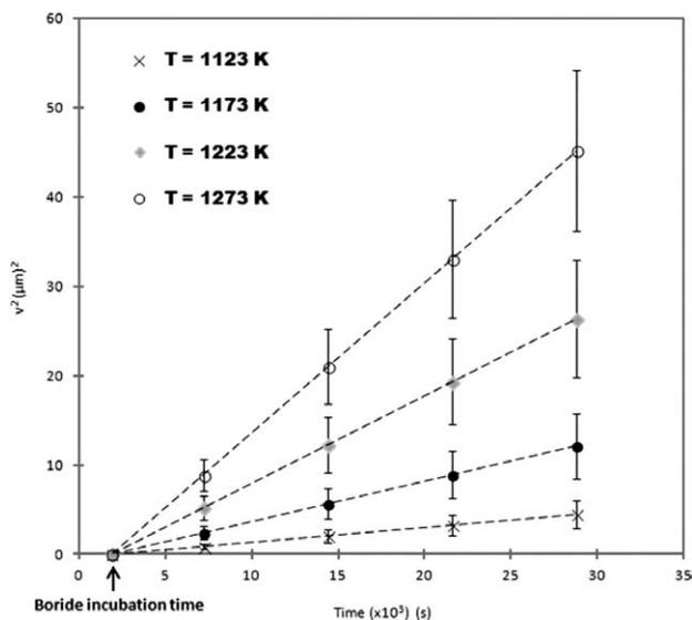
**Figure 13:** Square of the Fe<sub>2</sub>B layers thickness ( $v^2$ ) versus boriding time ( $t$ ) at different temperatures
