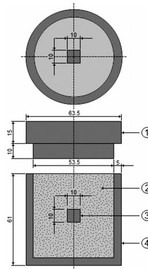
**Figure 5:** Schematic view of the stainless steel AISI 304L container for the powder-pack boriding treatment: 1 – lid; 2 – powder boriding medium (B<sub>4</sub>C + KBF<sub>4</sub> + SiC); 3 – sample; 4 – container
