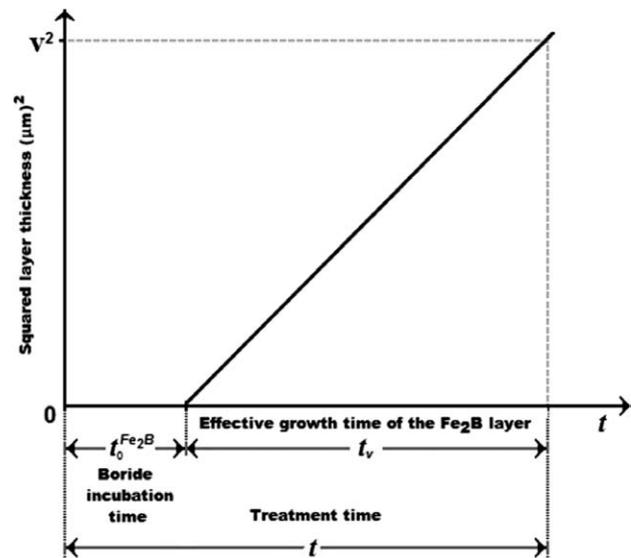
**Figure 3:** Schematic representation of the square of the Fe<sub>2</sub>B layer thickness against the treatment time
