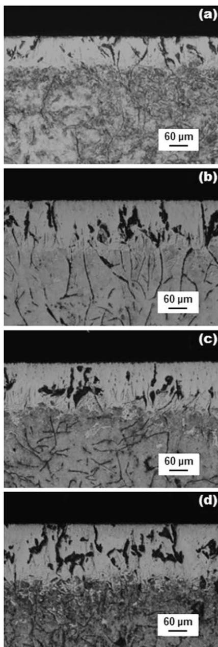
**Figure 7:** Light micrographs of the Fe<sub>2</sub>B layers formed at the surface of the borided ASTM A-48 alloy at 1223 K with the exposure times of: a) 2 h, b) 4 h, c) 6 h and d) 8 h
