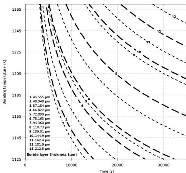
**Figure 16:** Contour diagram for the estimation of process parameters and layer thickness
