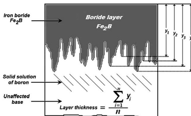
**Figure 8:** Schematic diagram illustrating the procedure of estimating the boride-layer thickness in gray cast iron
