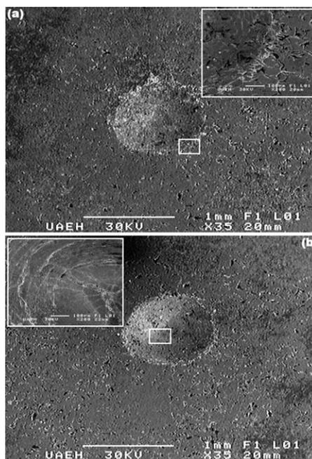
**Figure 12:** SEM micrographs: a) adjacent to the boundary of the indentation and b) center of the indentation of the VDI adhesion test on gray cast iron
