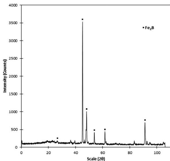
**Figure 10:** XRD patterns obtained for the surface of the borided ASTM A-48 gray cast iron at 1273 K after 8 h of treatment
