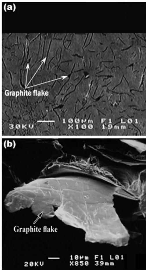
**Figure 4:** a) Microstructure of gray cast iron after solution treatment, b) SEM micrograph of a graphite flake
