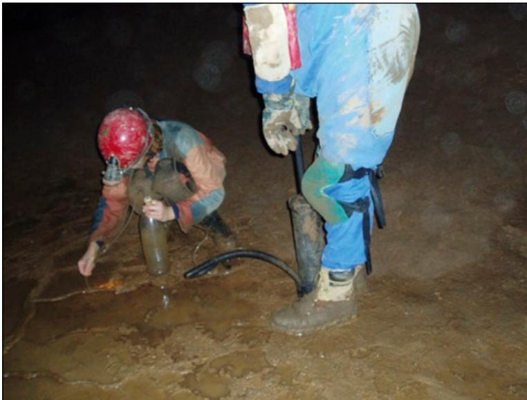
Figure 8.4: Apparatus for aspirating water in pools. After aspiration, the water is filtered through a net or filtering bottle (Fig. 8.3) in order to recover the epikarst fauna (Photo: Daniel W. Fong).
