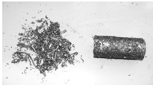
Figure 2: Separated stainless steel chips and compacted, cold pressed chips
