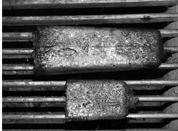
**Figure 6:** Ingots composed of basic steel and added compacts
