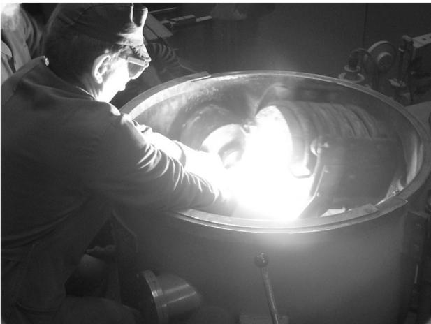
**Figure 5:** Casting of sample for chemical analysis
