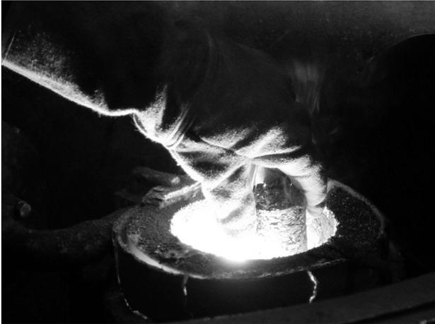
**Figure 4:** Charging of compact into melt
