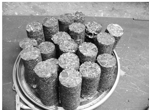
Figure 3: Compacts of stainless steel chips after cold pressing
