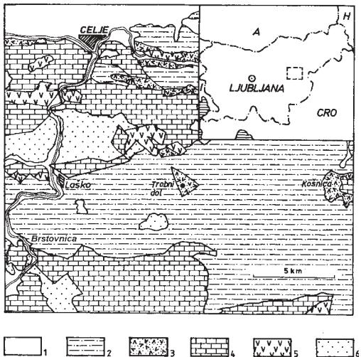
Fig. 1. Simplified geological map of the Trobni Dol area (modified after Buser 1977). 1, Quaternary; 2, Mio-Pliocene clay, silt, sand and gravel; 3, Oligocene volcaniclastics; 4, Mesozoic carbonates; 5, triassic keratophyre and tuffs; 6, Permian and Carboniferous clastic rocks
