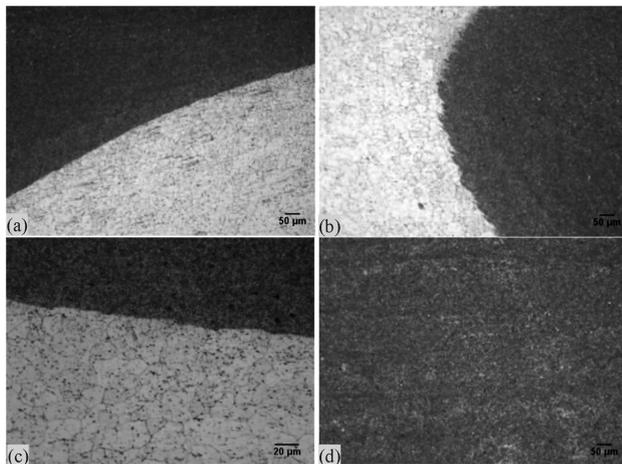
**Figure 8:** Microstructure of various regions of sample processed with 20 mm tool shoulder diameter showing: a) AS interface, b) RS interface, c) bottom interface and d) SZ
