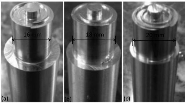
**Figure 3:** FSP tools having shoulder diameter: a) 16 mm, b) 18 mm, and c) 20 mm
