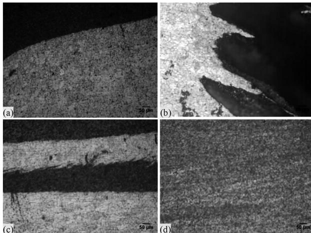
**Figure 7:** Microstructure of various regions of sample processed with 18 mm tool shoulder diameter showing: a) AS interface, b) agglomerated region in RS side, c) bottom interface and d) SZ
