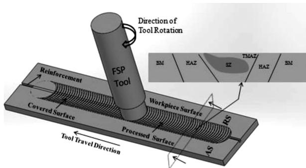
**Figure 1:** Schematic diagram of FSP
