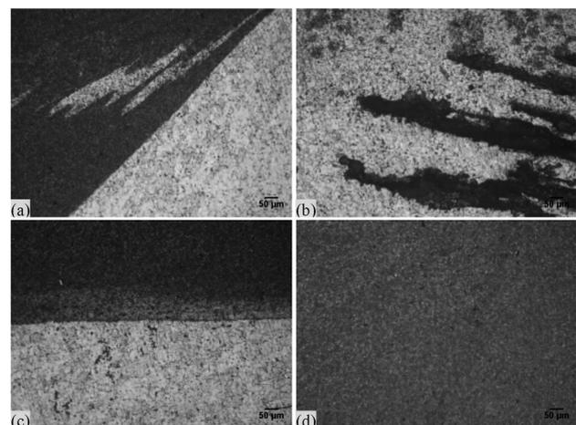
**Figure 6:** Microstructure of various regions of sample processed with 16 mm tool shoulder diameter showing: a) AS interface, b) agglomerated region in RS side, c) bottom interface and d) SZ
