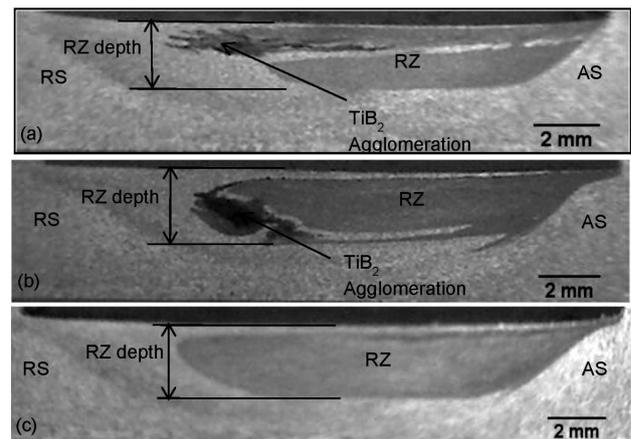
**Figure 5:** Macrograph of cross-section of PZ processed with tool shoulder diameter of: a) 16 mm, b) 18 mm and c) 20 mm
