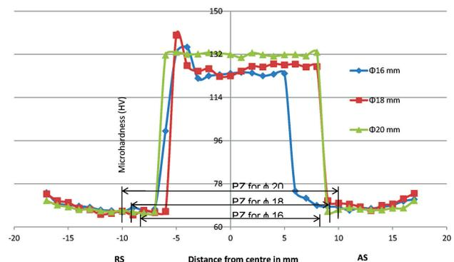
**Figure 9:** Hardness profiles
