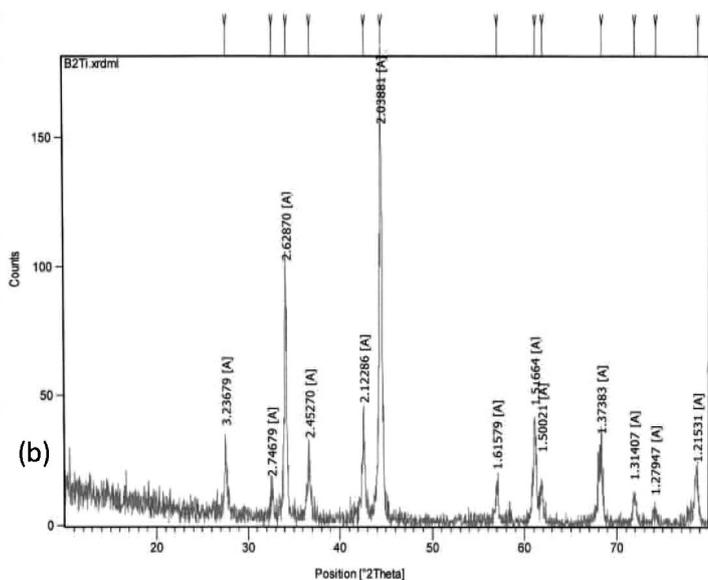
**Figure 2:** a) SEM micrograph, and b) XRD pattern of titanium diboride (TiB<sub>2</sub>) nano powder
