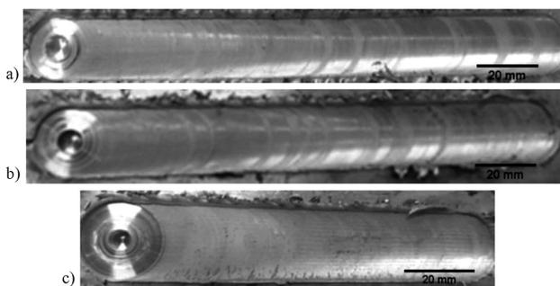
**Figure 4:** Friction stir processed plates with tool shoulder diameter of: a) 16 mm, b) 18 mm, and c) 20 mm
