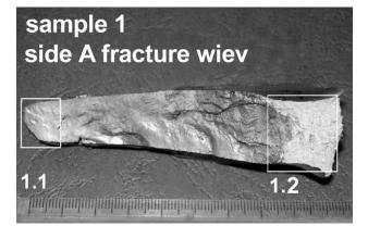
Figure 9: Side-A fracture surface of sample 1 Slika 9: Površina preloma na strani A vzorca 1
