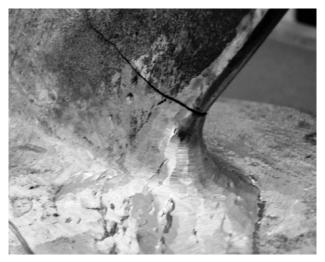
**Figure 5:** Crack at the leading edge of the blade **Slika 5:** Razpoka na vodilnem robu lopatice
