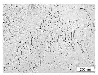
Figure 7: As-cast microstructure of the hub-to-blade attachment Slika 7: Mikrostruktura ulitka na stiku pesta in lopatice
