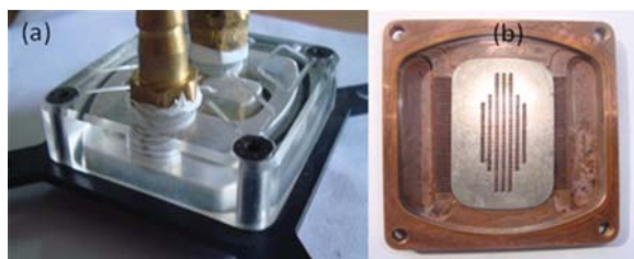
Fig. 6. a) Photograph of heat sink, and b) thin-channelled copper base with jet plate [18]
