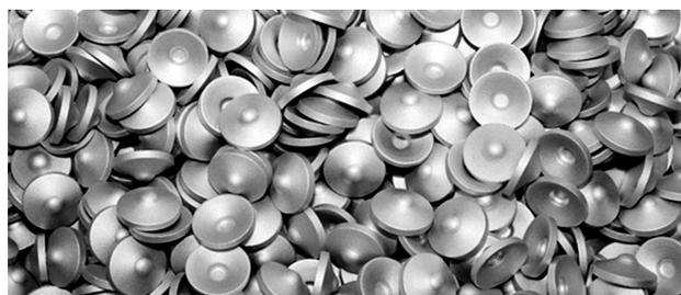
**Figure 3:** Slugs produced in the Talum Al factory used as semi-products in the production of tubes and containers in the pharmaceutical, food and cosmetic industries<sup>8</sup>
