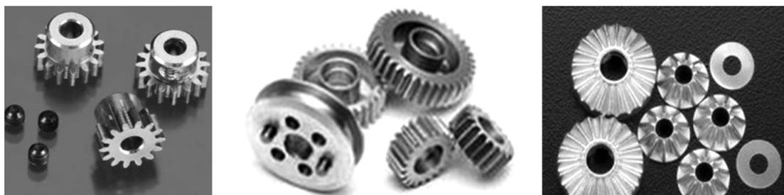
**Figure 2:** Some small complex Al-based sintered parts<sup>4</sup>
