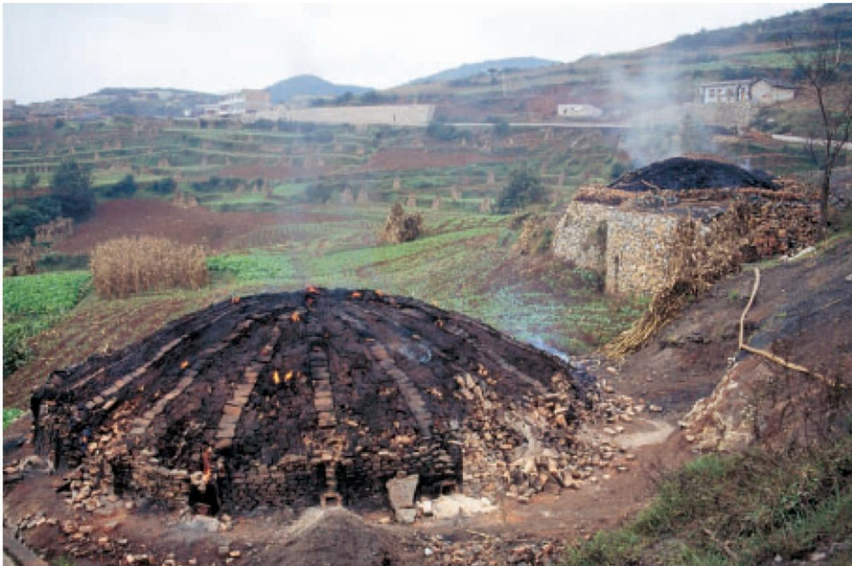
*Fig. 2.10.15. Pile for producing coke. The escape of gases rich in sulfur oxides is visible. (Photo A. Mihevc)*
