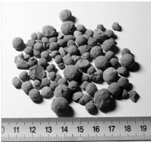
**Figure 2:** Granulometry of the synthetic slag REFRAFLUX 4842 S
